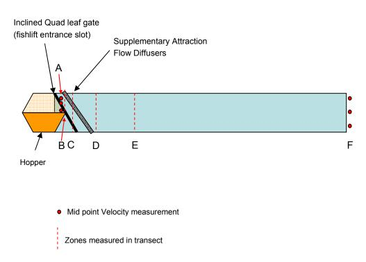
Figure 11 Side view of fishlift approach channel and locations of measurement transects
