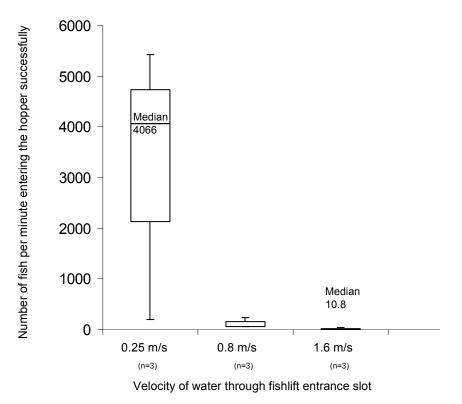
**Figure 16** Box and whisker plots demonstrating data distributions of the number of fish identified during different flow release treatments through the Paradise Dam fishlift entrance slot.
