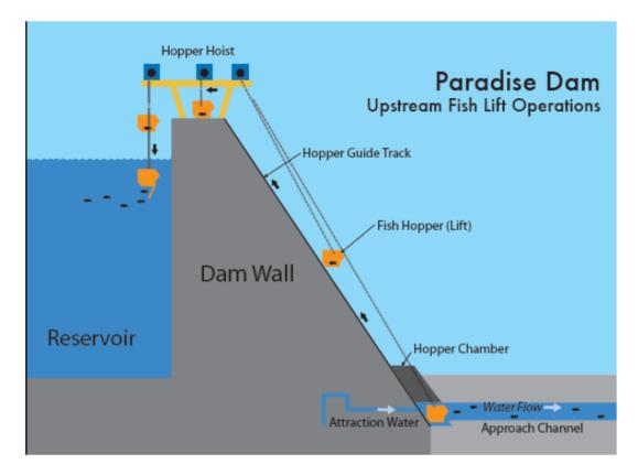
Figure 4 Schematic of the upstream fishlift at the Paradise Dam.
