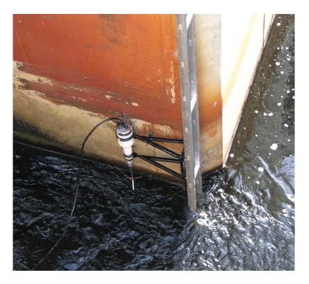
**Figure 10** ADV mounted on an adjustable frame for measuring hydraulic conditions within the fishway.
