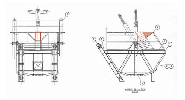
**Figure 25** Diagram showing proposed hopper cone entrance modifications that will allow the hopper to be lowered further into the hopper chamber.
