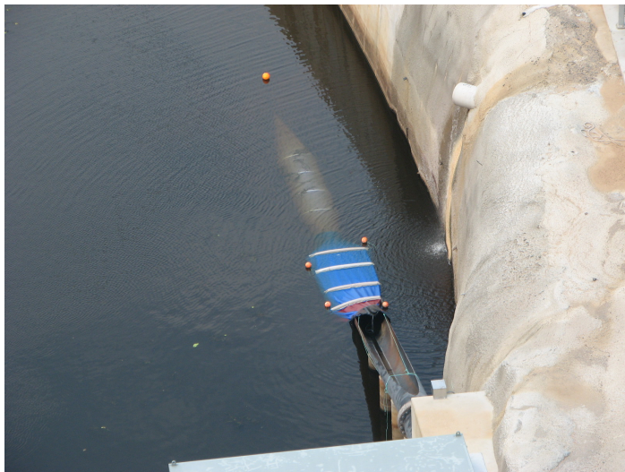
Figure 6 The exit chute sampling net at the downstream fishway exit chute.
