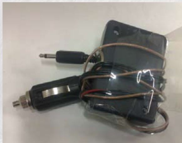
Picture of a device for forging tachograph charts which is connected to the tachograph and the cigarette lighter of a vehicle.
