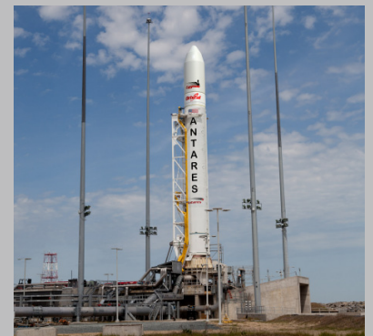
Cygnus will be boosted into orbit by Orbital's Antares medium-class space launch vehicle.
