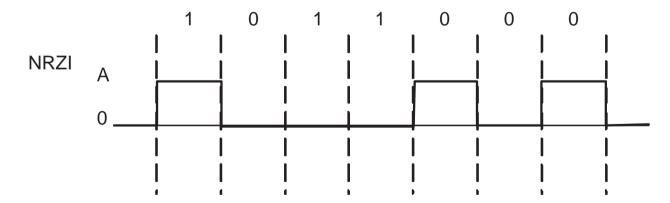
In 4B/5B coding, as only 16 of the 32 pulse patterns are used to encode 4 bits, 5—pulse codes can be selected in such a way that at least 2 transitions are present in each pulse pattern. The diagram below illustrates 4B/5B NRZI coding. Note that that in the NRZI code used here a 1 represents a change of state and a 0 represents the absence of a change of state.
