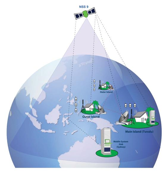
The Tuvalu mobile system contains a local controller and is completely autonomous. It is directly connected to the International and Domestic Public Service Telephone Network and all calls are switched locally. Equipment providing complex services such as billing, roaming and international SMS is installed in Pactel's Sydney data centre. Load testing, failover and disaster recovery have been performed to ensure that the system works as designed.
