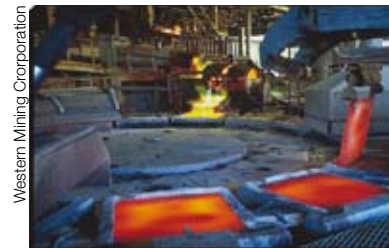
Western Mining Corporation Casting copper anodes in the Olympic Dam smelter
