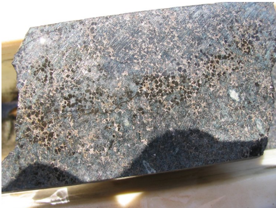
Figure 9: Photograph of core showing net-textured magmatic sulphides (pyrrhotite \pm pentlandite & chalcopyrite) associated with cumulate textured olivine grains. Core diameter is NQ2.
