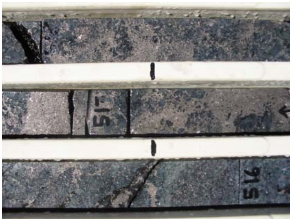
Figure 10: Photograph of core showing semi-massive pyrrhotite (with minor pentlandite and chalcopyrite) within gabbro-norite (SMD02: 516m to 518m). Core diameter is NQ2.
