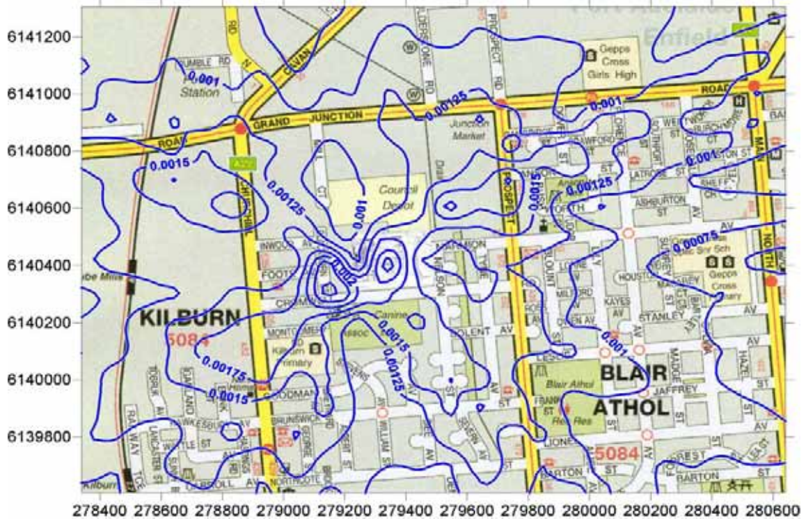
Figure 15: Predicted furane based phenol GLC from future (furane) operation (mg/m3). (3 minute averaging period, 100th percentile)
