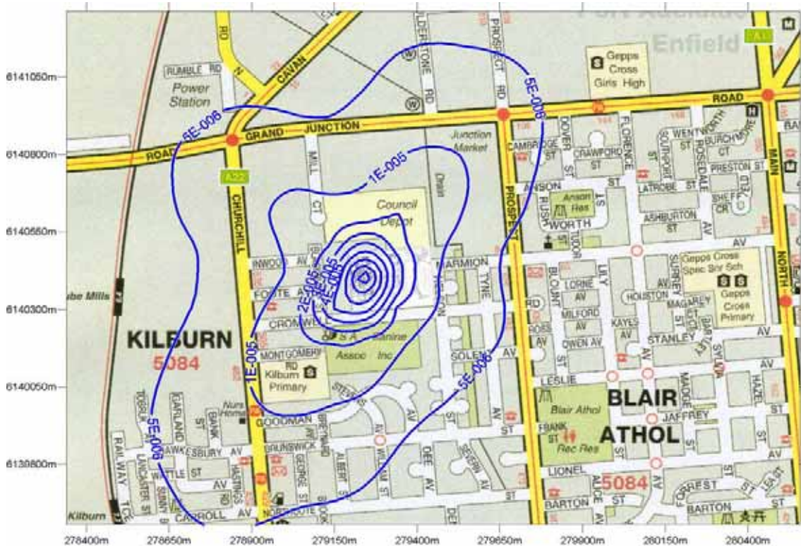
Figure 30: Predicted styrene GLC from future (furane) operation ( \text{mg}/\text{m}^3 ). (Annual averaging period, 100 th percentile)
