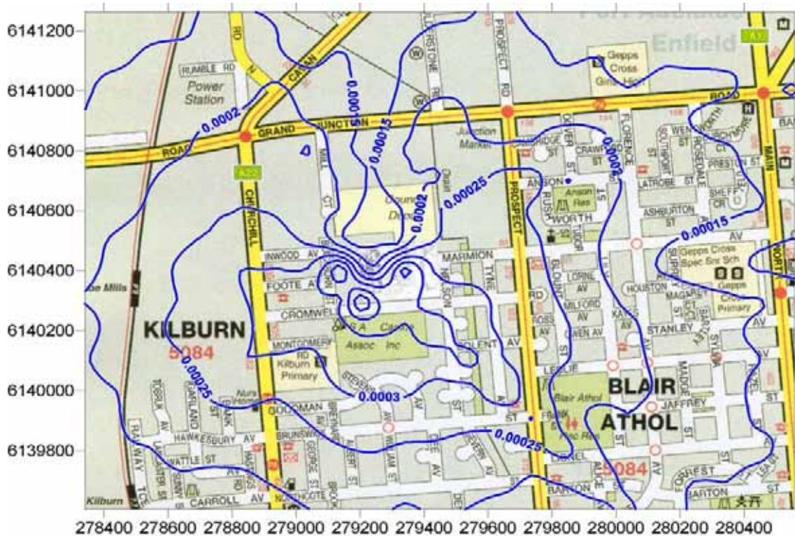
Figure 37: Predicted pentanaldehyde GLC from existing operation (mg/m 3 ). (3 minute averaging period, 100 th percentile)
