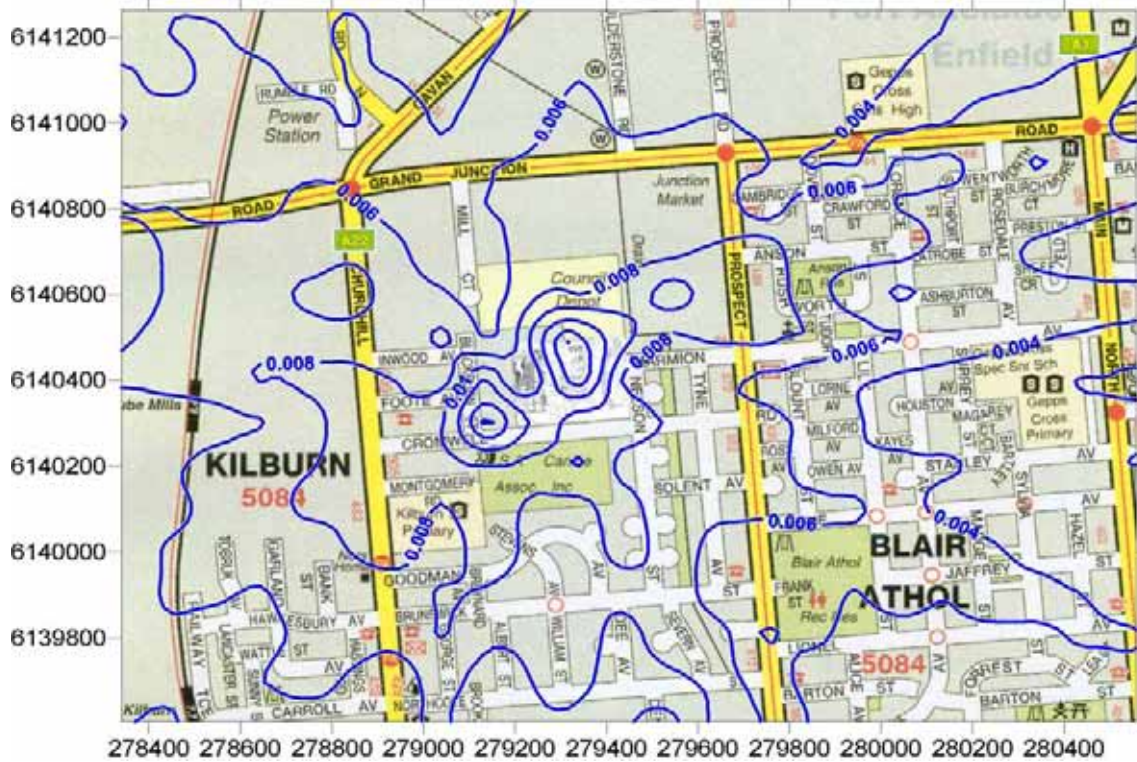
Figure 3: Predicted hydrogen sulphide GLC from future (furane) operation (mg/m3). (3 minute averaging period, 100th percentile)
