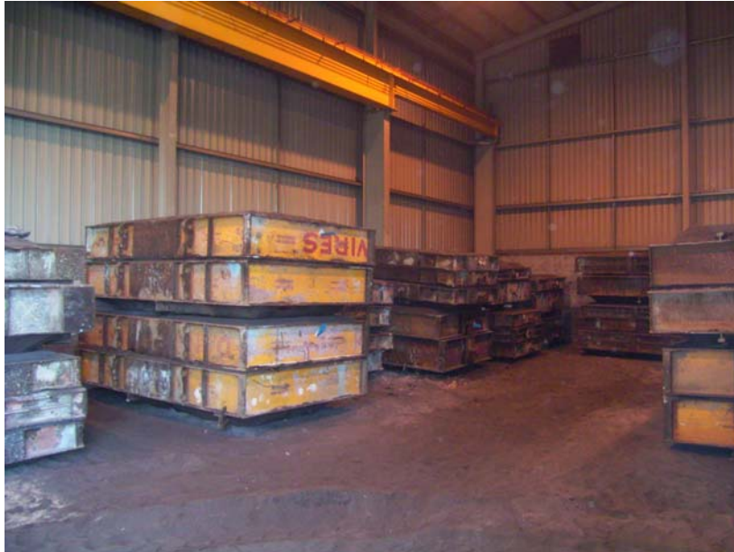
Figure 8: Poured moulds are stored for cooling, nominally up to 48 hours before knockout
