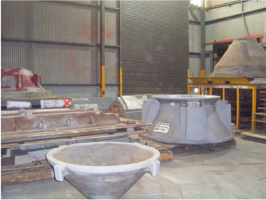
Figure 4: Timber patterns are used to produce a cavity in the sand moulds and are a replica of the steel casting to be produced
