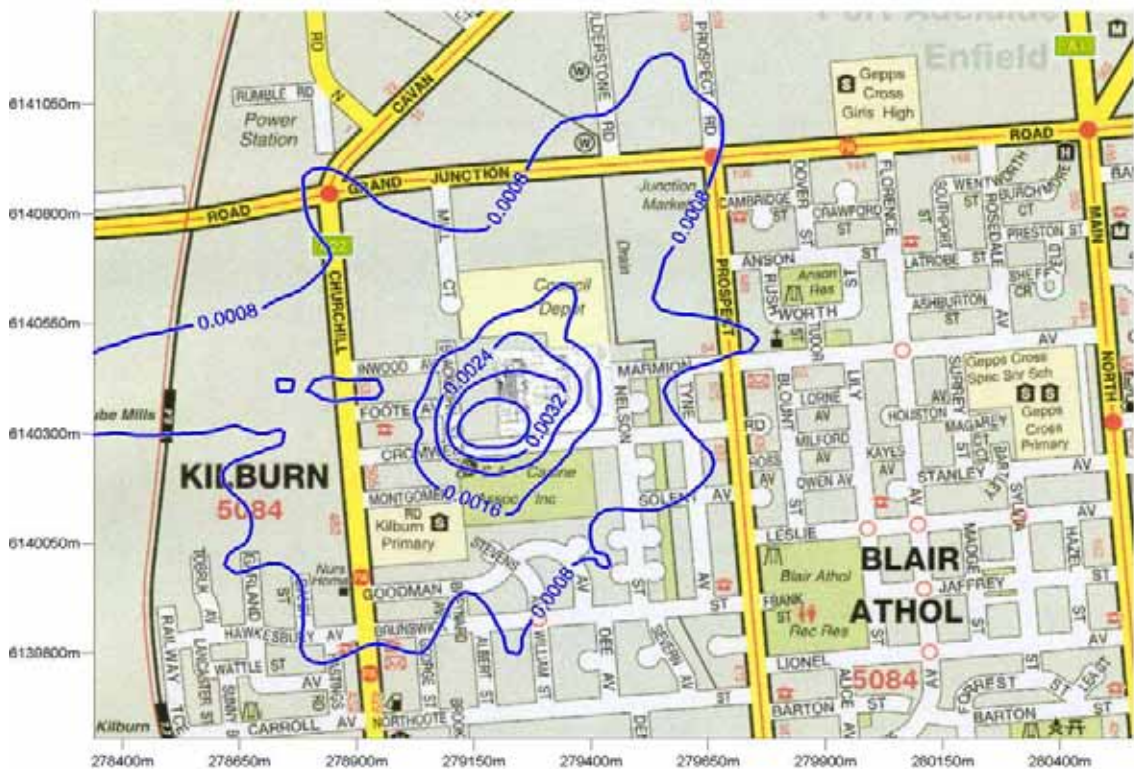
Figure 32: Predicted acetaldehyde GLC from future (furane) operation ( \text{mg}/\text{m}^3 ). (24 hour averaging period, 100 th percentile)
