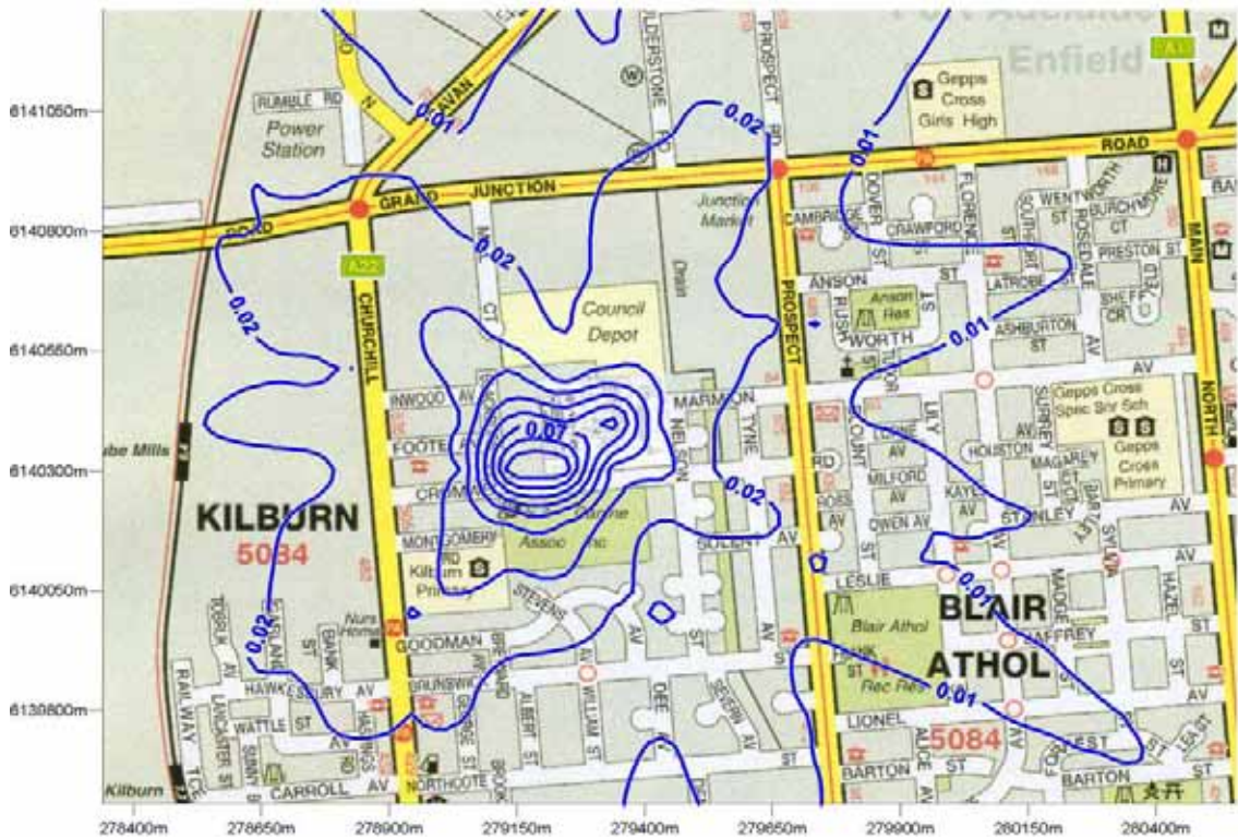
Figure 14: Predicted toluene GLC from future (furane) operation ( \text{mg}/\text{m}^3 ). (24 hour averaging period, 100 th percentile)
