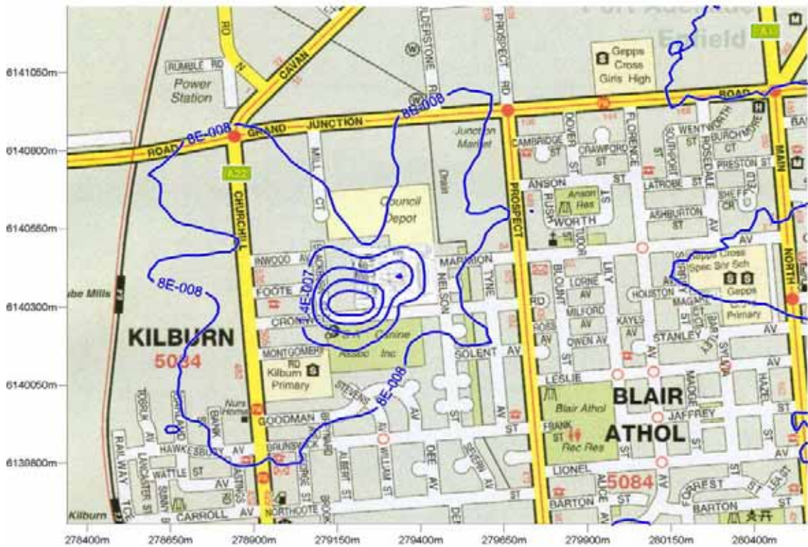
Figure 44: Predicted chrysene GLC from future (furane) operation ( \text{mg}/\text{m}^3 ). (24 hour averaging period, 100 th percentile)
