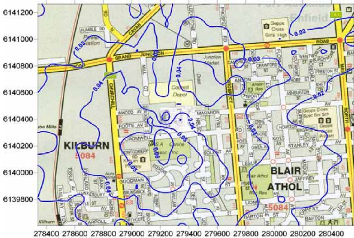
Figure 9: Predicted benzene GLC from existing operation ( \text{mg}/\text{m}^3 ). (3 minute averaging period, 100 th percentile)
