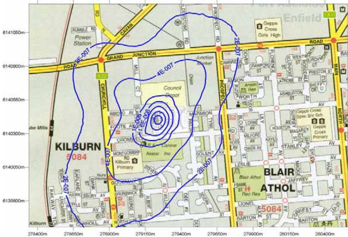
Figure 28: Predicted phenanthrene GLC from future (furane) operation ( \text{mg}/\text{m}^3 ). (Annual averaging period, 100 th percentile)
