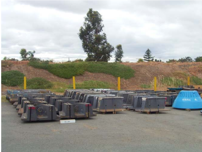
Figure 11: Castings are made ready for despatch after dressing, some are also machined and painted before despatch
