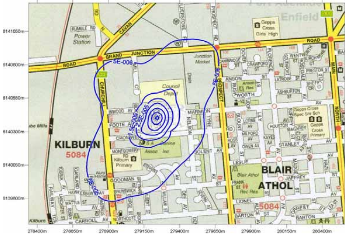
Figure 21: Predicted cyclohexanone GLC from future (furane) operation ( \text{mg}/\text{m}^3 ). (Annual averaging period, 100 th percentile)
