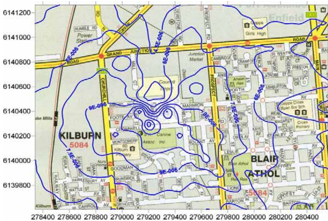
Figure 30: Predicted pyrene GLC from existing operation ( \text{mg}/\text{m}^3 ). (3 minute averaging period, 100 th percentile)
