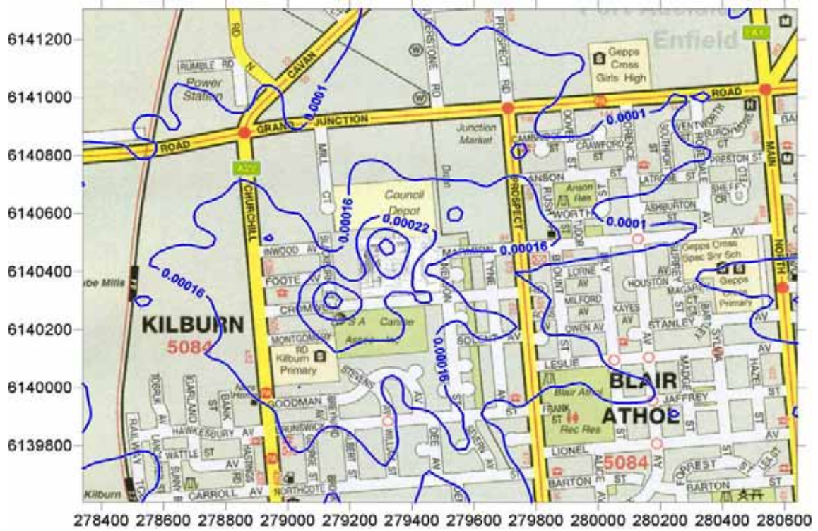
Figure 17: Predicted acrolein GLC from future (furane) operation (mg/m3). (3 minute averaging period, 100th percentile)
