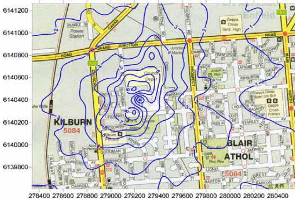
Figure 3: Predicted odour GLC from existing operation (ODU). (3 minute averaging period, 99.9 th percentile)
