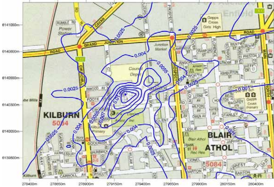
Figure 5: Predicted nitrogen oxides GLC from future (furane) operation ( \mu\text{g}/\text{m}^3 ). (24 hour averaging period, 100 th percentile)
