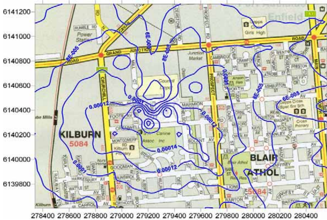
Figure 17: Predicted anthracene GLC from existing operation ( \text{mg}/\text{m}^3 ). (3 minute averaging period, 100 th percentile)
