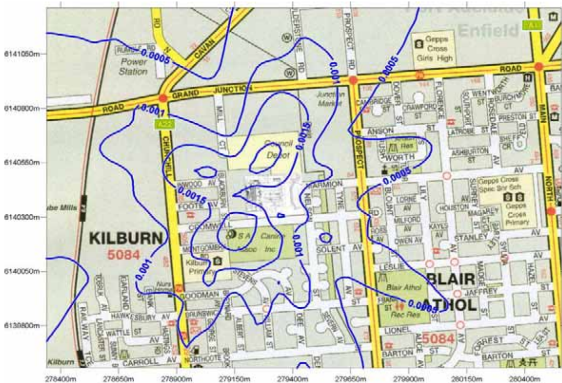
Figure 8: Predicted benzene GLC from future (furane) operation ( \text{mg}/\text{m}^3 ). (24 hour averaging period, 100 th percentile)
