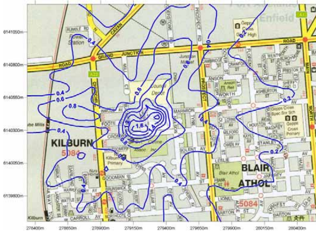
Figure 47: Predicted CO GLC from future operation (mg/m 3 ). (8 hour averaging period, 100th percentile)
