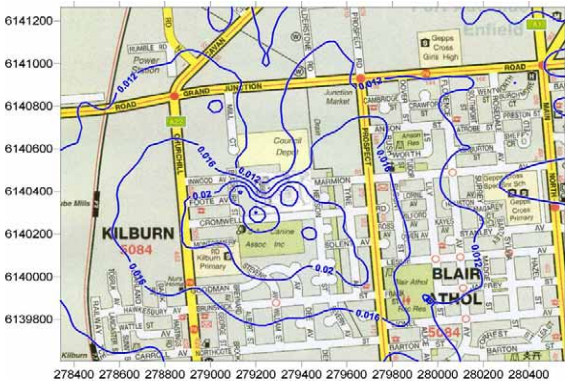
Figure 46: Predicted dimethylphenols GLC from existing operation ( \text{mg}/\text{m}^3 ). (3 minute averaging period, 100 th percentile)
