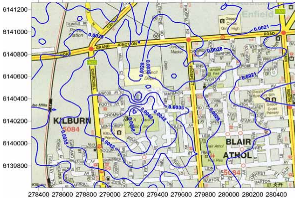
Figure 11: Predicted cyanide GLC from existing operation ( \text{mg}/\text{m}^3 ). (3 minute averaging period, 100 th percentile)
