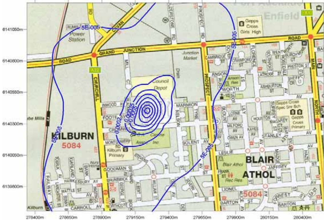
Figure 9: Predicted formaldehyde GLC from future (furane) operation ( \text{mg}/\text{m}^3 ). (Annual averaging period, 100 th percentile)
