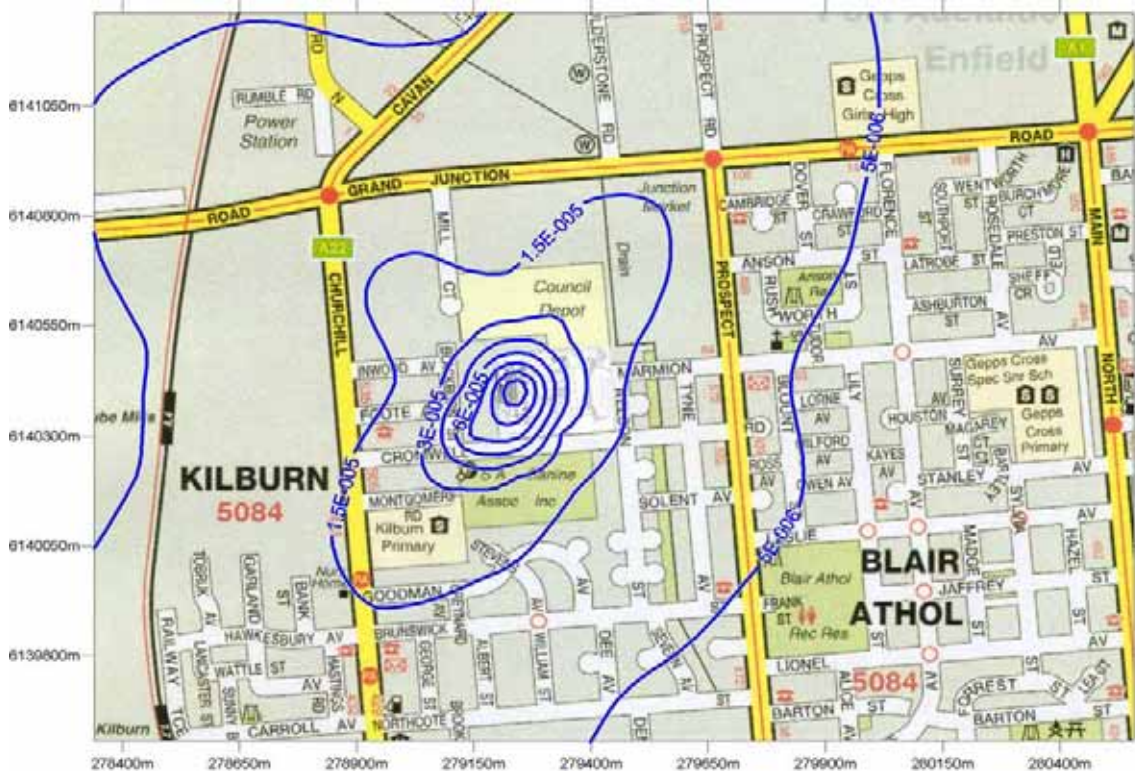
Figure 23: Predicted ethyl benzene GLC from future (furane) operation ( \text{mg}/\text{m}^3 ). (Annual averaging period, 100 th percentile)
