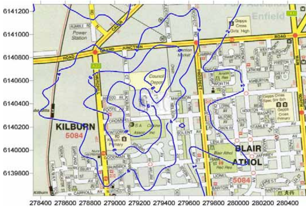
Figure 7: Predicted PM 2.5 GLC from existing operation (µg/m 3 ). (24 hour averaging period, 100 th percentile)
