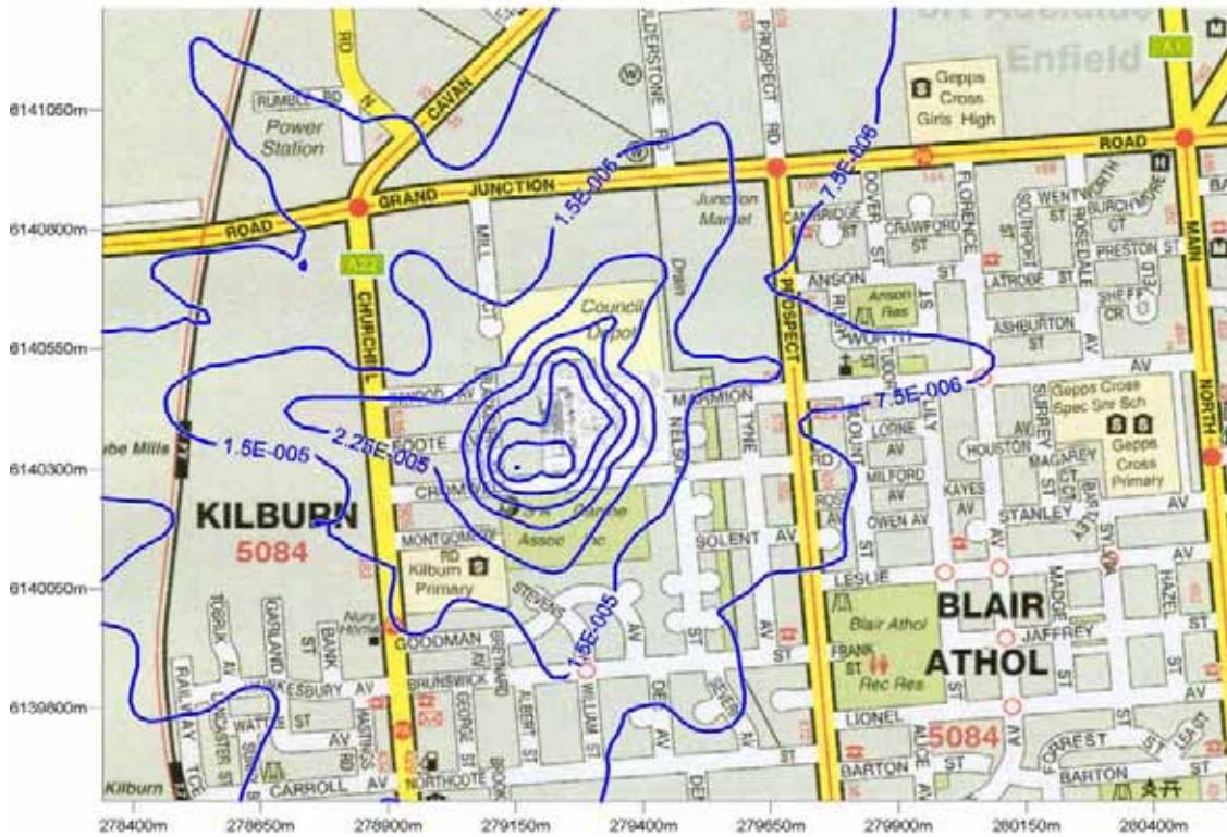
Figure 15: Predicted acrolein GLC from future (furane) operation ( \text{mg}/\text{m}^3 ). (24 hour averaging period, 100 th percentile)
