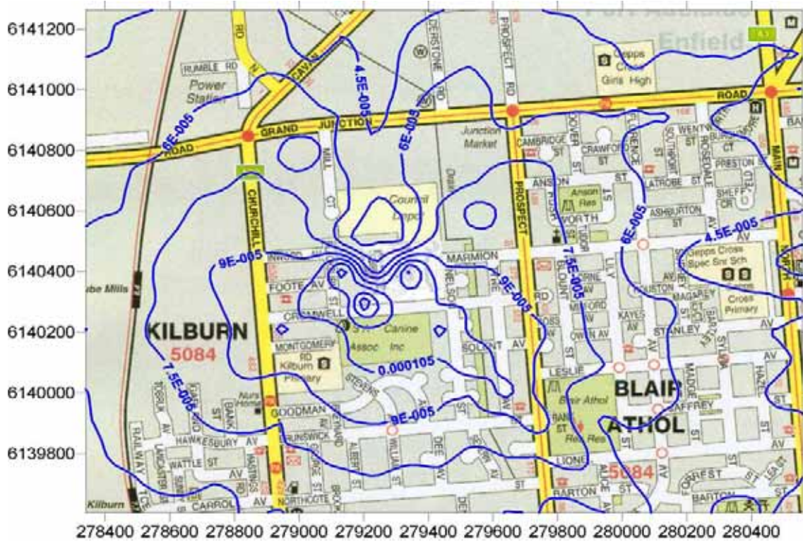
Figure 25: Predicted fluorene GLC from existing operation ( \text{mg}/\text{m}^3 ). (3 minute averaging period, 100 th percentile)
