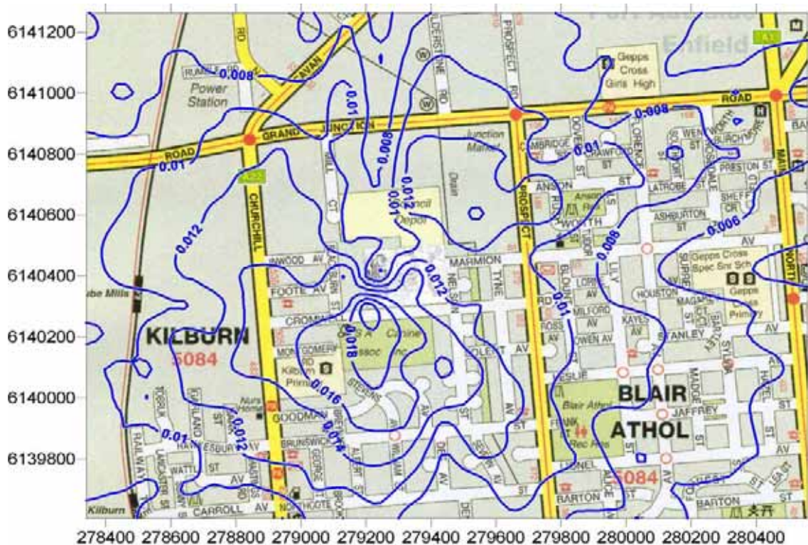
Figure 10: Predicted formaldehyde GLC from existing operation ( \text{mg}/\text{m}^3 ). (3 minute averaging period, 100 th percentile)
