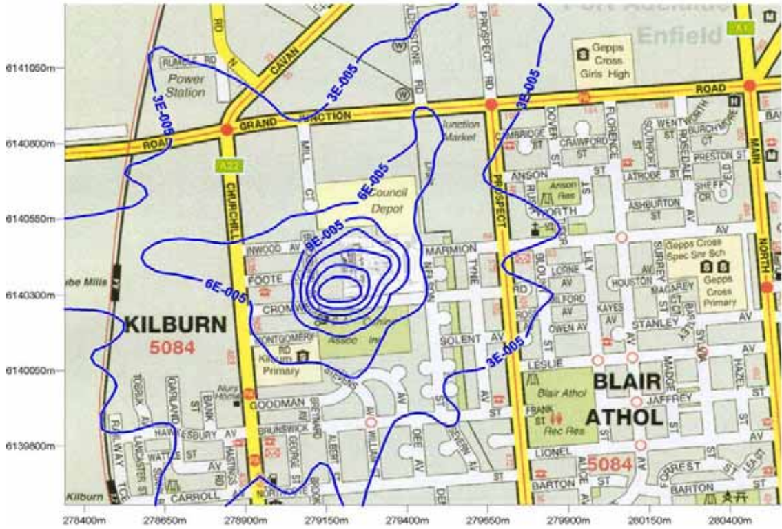
Figure 27: Predicted methylisobutylketone GLC from future (furane) operation ( \text{mg}/\text{m}^3 ). (24 hour averaging period, 100 th percentile)
