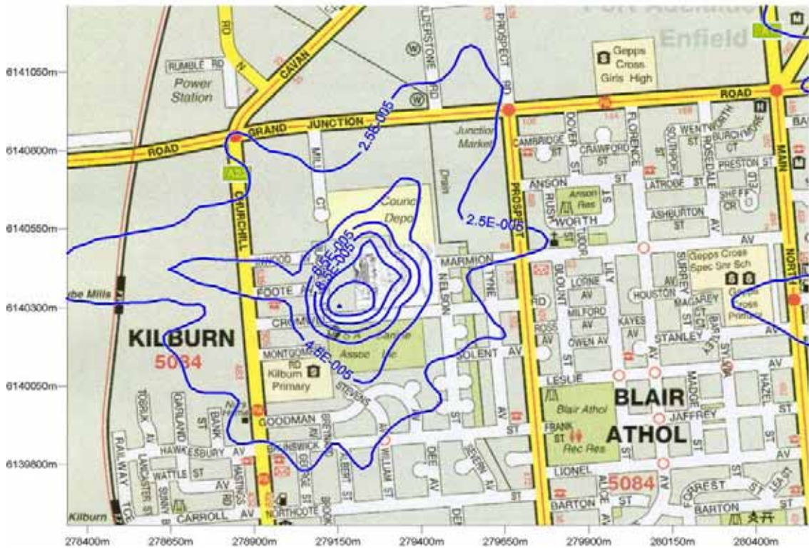
Figure 31: Predicted butanol GLC from future (furane) operation ( \text{mg}/\text{m}^3 ). (24 hour averaging period, 100 th percentile)
