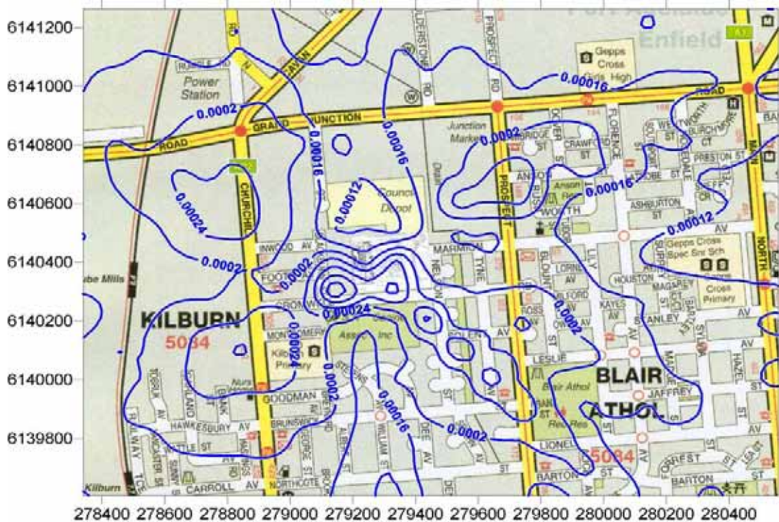
Figure 38: Predicted pentanaldehyde GLC from future (furane) operation (ug/m3). (3 minute averaging period, 100th percentile)
