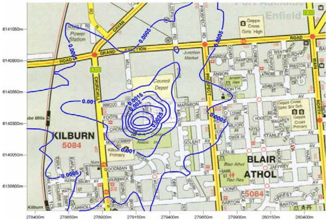
Figure 2: Predicted hydrogen sulphide GLC from future (furane) operation ( \text{mg}/\text{m}^3 ). (24 hour averaging period, 100 th percentile)
