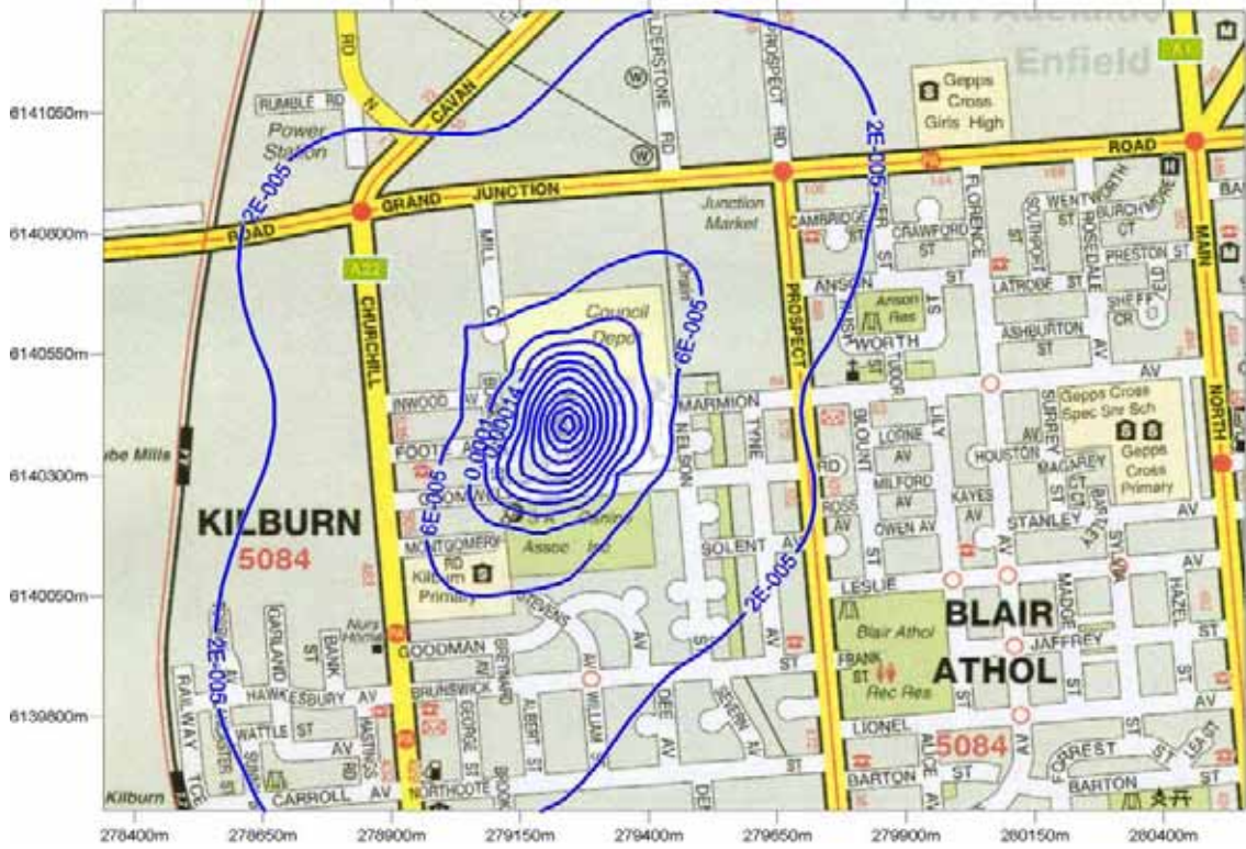
Figure 1: Predicted ammonia GLC from future (furane) operation ( \text{mg}/\text{m}^3 ). (Annual averaging period, 100 th percentile)
