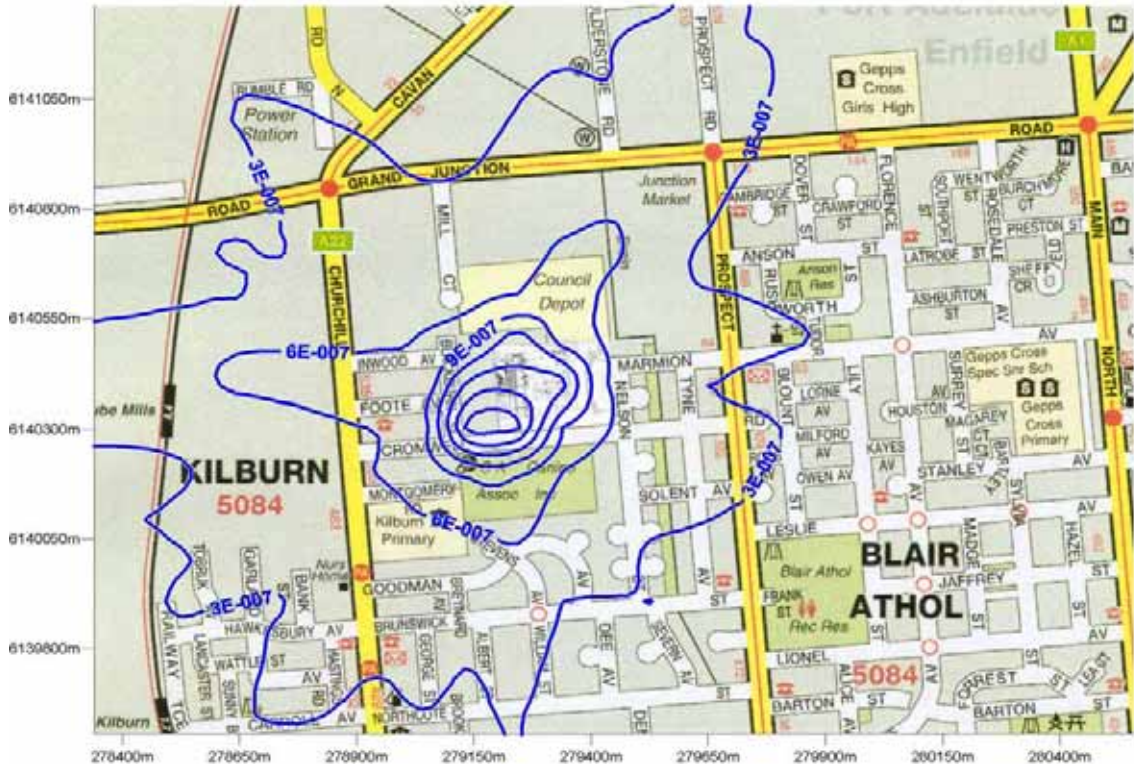
Figure 29: Predicted pyrene GLC from future (furane) operation ( \text{mg}/\text{m}^3 ). (24 hour averaging period, 100 th percentile)
