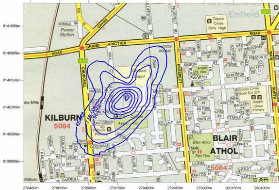
Figure 40: Predicted acenaphthylene GLC from future (furane) operation ( \text{mg}/\text{m}^3 ). (Annual averaging period, 100 th percentile)
