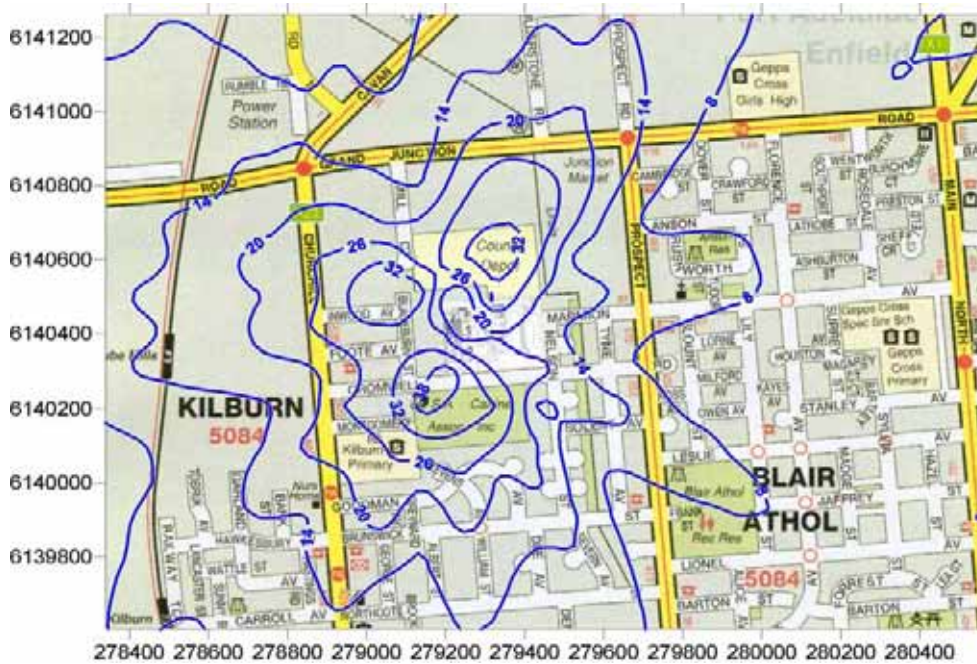
Figure 5: Predicted PM 10 GLC from existing operation ( \mu\text{g}/\text{m}^3 ). (24 hour averaging period, 100 th percentile)
