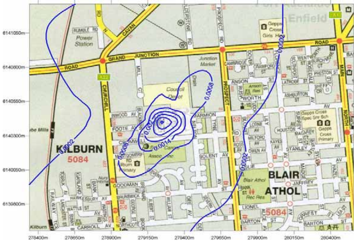
Figure 5: Predicted nitrogen oxides GLC from future (furane) operation ( \mu\text{g}/\text{m}^3 ). (Annual averaging period, 100 th percentile)
