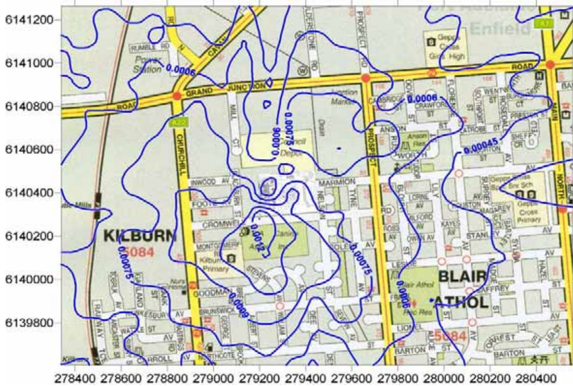
Figure 27: Predicted methylethylketone GLC from existing operation ( \text{mg}/\text{m}^3 ). (3 minute averaging period, 100 th percentile)
