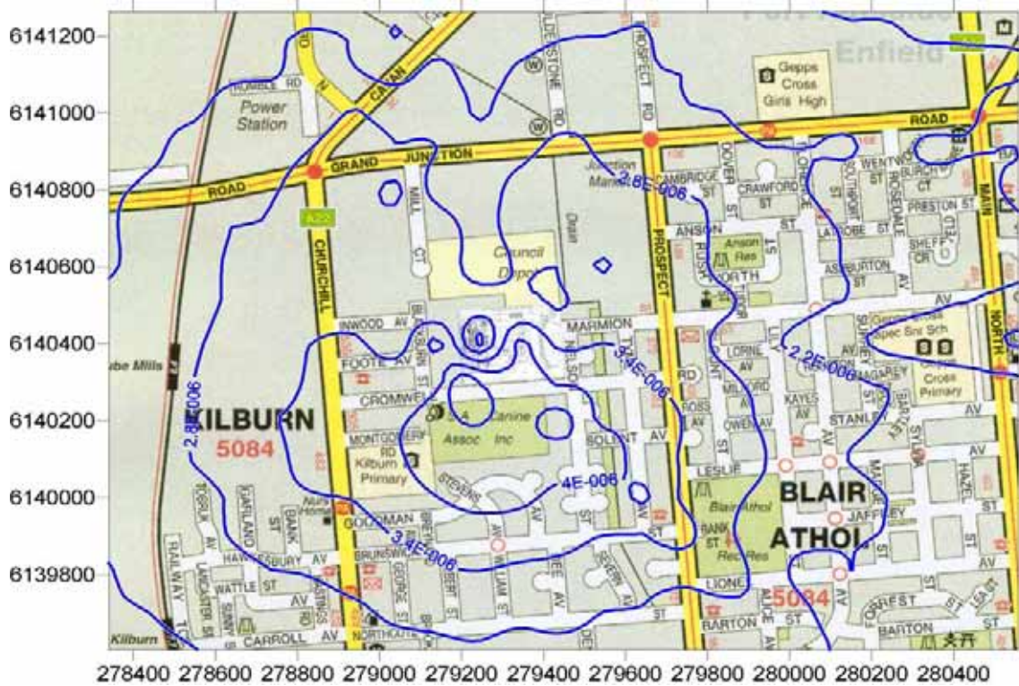
Figure 42: Predicted benz(a)anthracene GLC from existing operation ( \text{mg}/\text{m}^3 ). (3 minute averaging period, 100 th percentile)
