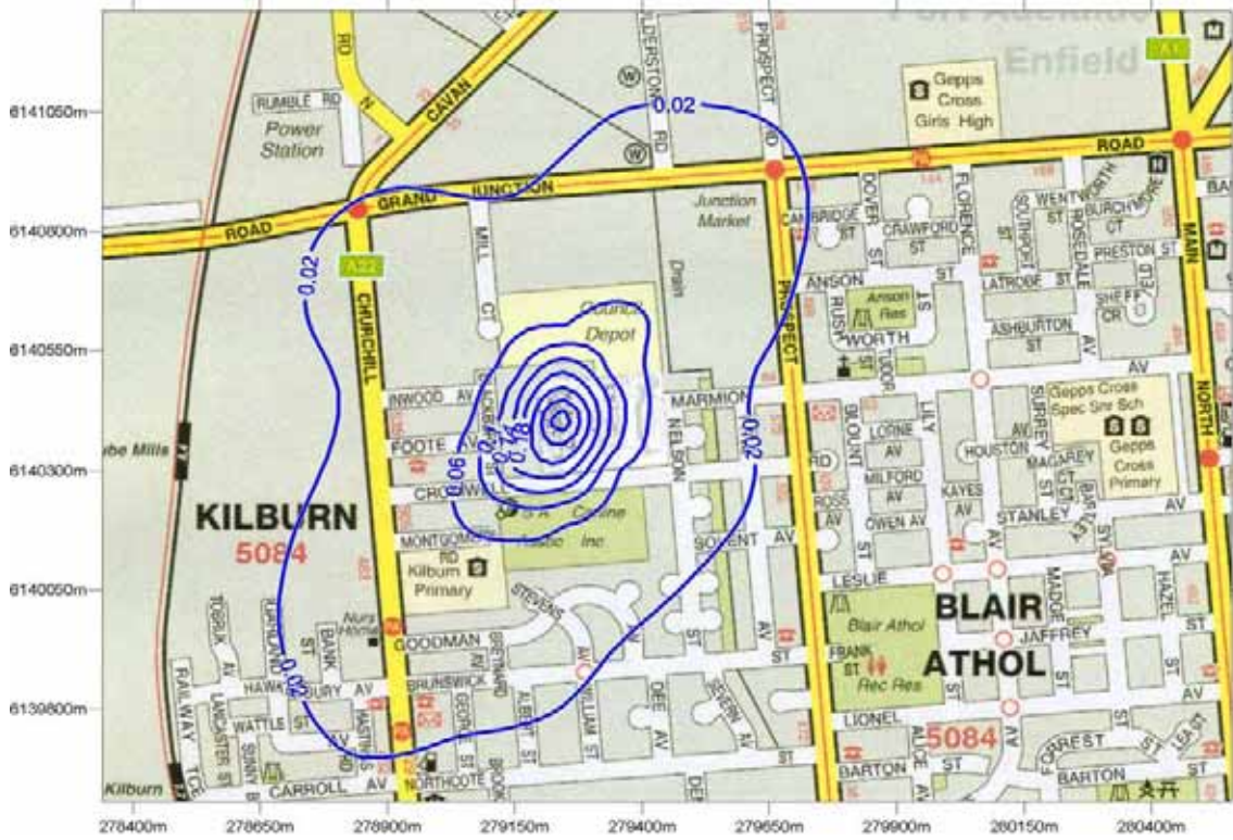
Figure 19: Predicted carbon monoxide GLC from future (furane) operation ( \text{mg}/\text{m}^3 ). (Annual averaging period, 100 th percentile)
