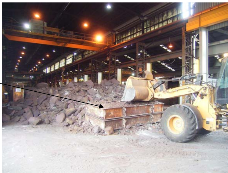
Figure 9: The steel castings are retrieved from the sand mould in the knockout area
