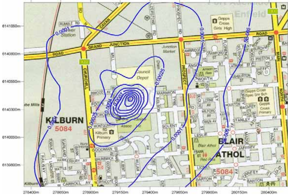
Figure 11: Predicted total xylene GLC from future (furane) operation ( \text{mg}/\text{m}^3 ). (Annual averaging period, 100 th percentile)
