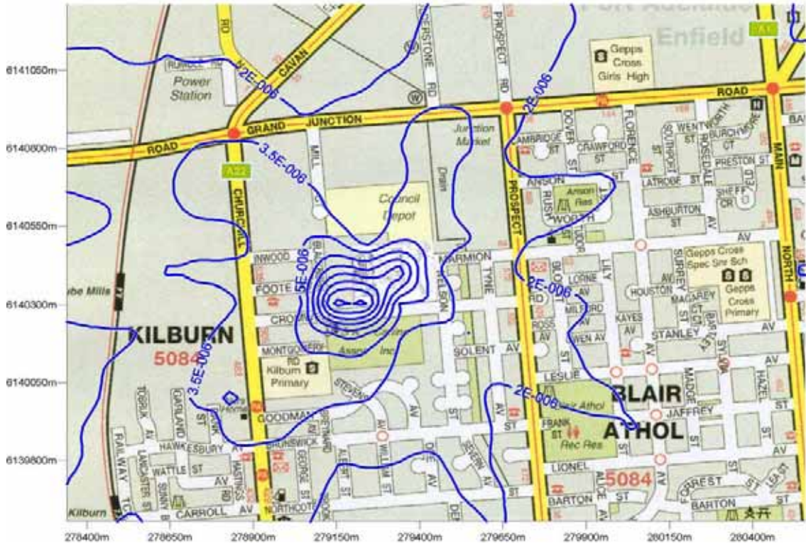
Figure 33: Predicted furfural GLC from future (furane) operation ( \mu\text{g}/\text{m}^3 ). (24 hour averaging period, 100 th percentile)
