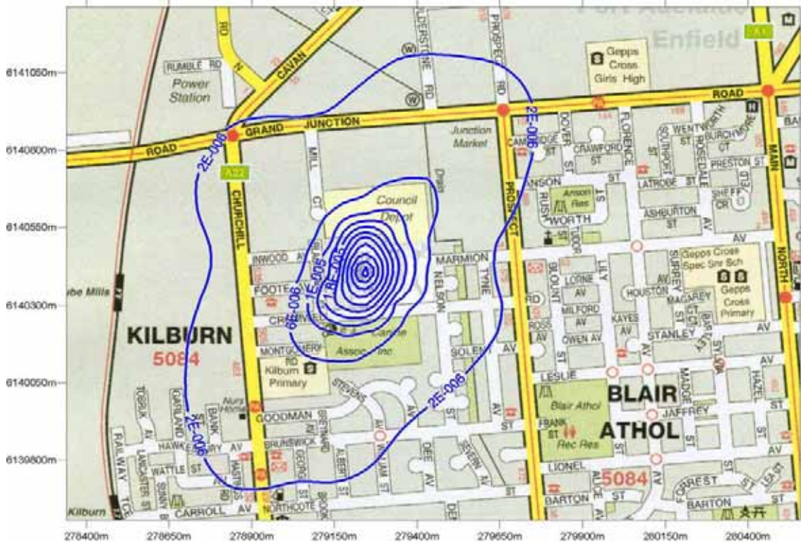
Figure 31: Predicted butanol GLC from future (furane) operation ( \text{mg}/\text{m}^3 ). (Annual averaging period, 100 th percentile)
