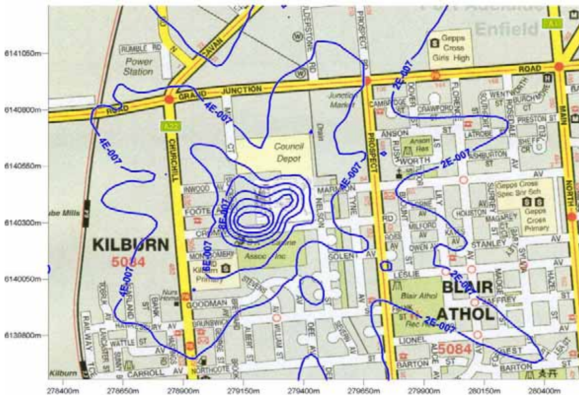
Figure 16: Predicted anthracene GLC from future (furane) operation ( \text{mg}/\text{m}^3 ). (24 hour averaging period, 100 th percentile)
