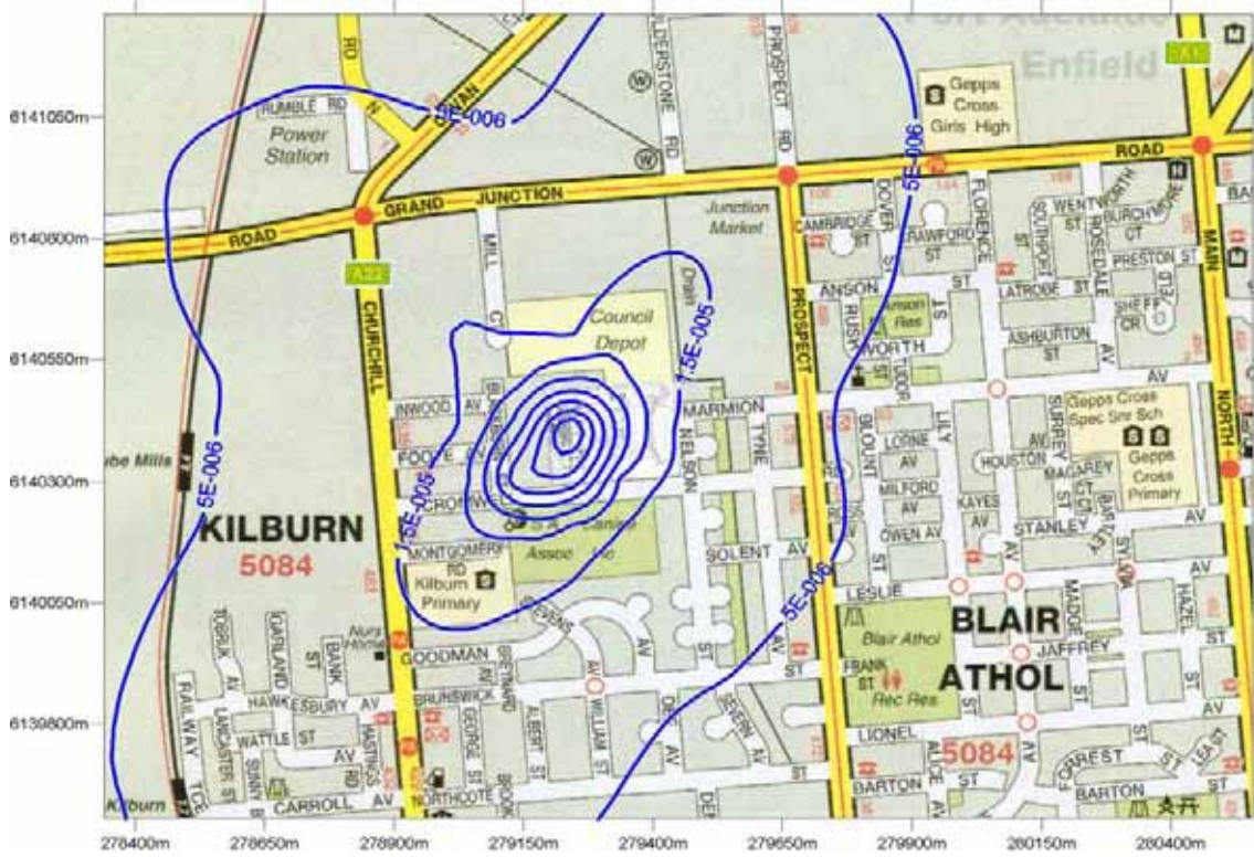
Figure 37: Predicted benzaldehyde GLC from future (furane) operation ( \text{mg}/\text{m}^3 ). (Annual averaging period, 100 th percentile)
