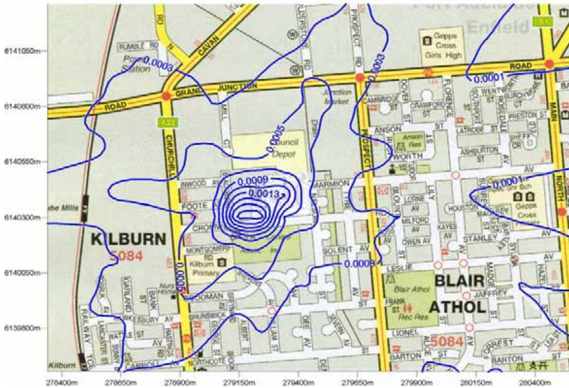
Figure 35: Predicted butanaldehyde GLC from future (furane) operation ( \text{mg}/\text{m}^3 ). (24 hour averaging period, 100 th percentile)
