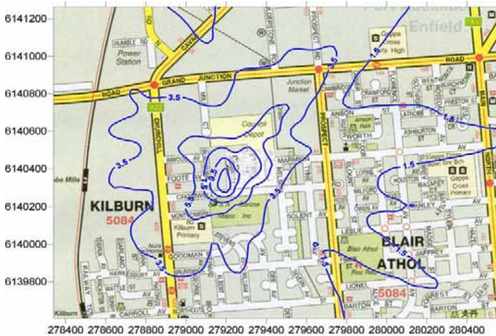
Figure 6: Predicted PM 10 GLC from future operation ( \mu\text{g}/\text{m}^3 ). (24 hour averaging period, 100 th percentile)
