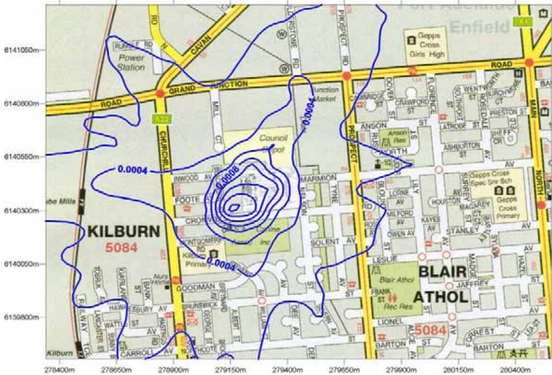
Figure 1: Predicted ammonia GLC from future (furane) operation ( \text{mg}/\text{m}^3 ). (24 hour averaging period, 100 th percentile)
