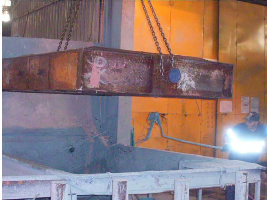
Figure 6: The sand moulds are coated with refractory paint to obtain a good surface finish on the castings
