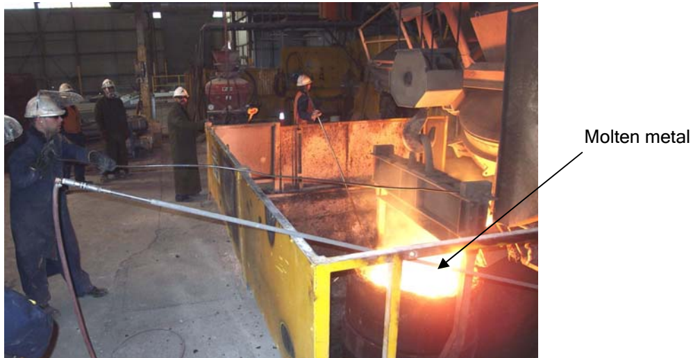
Figure 3: Molten metal from the furnace is tapped into a ladle for transport to the waiting sand moulds
