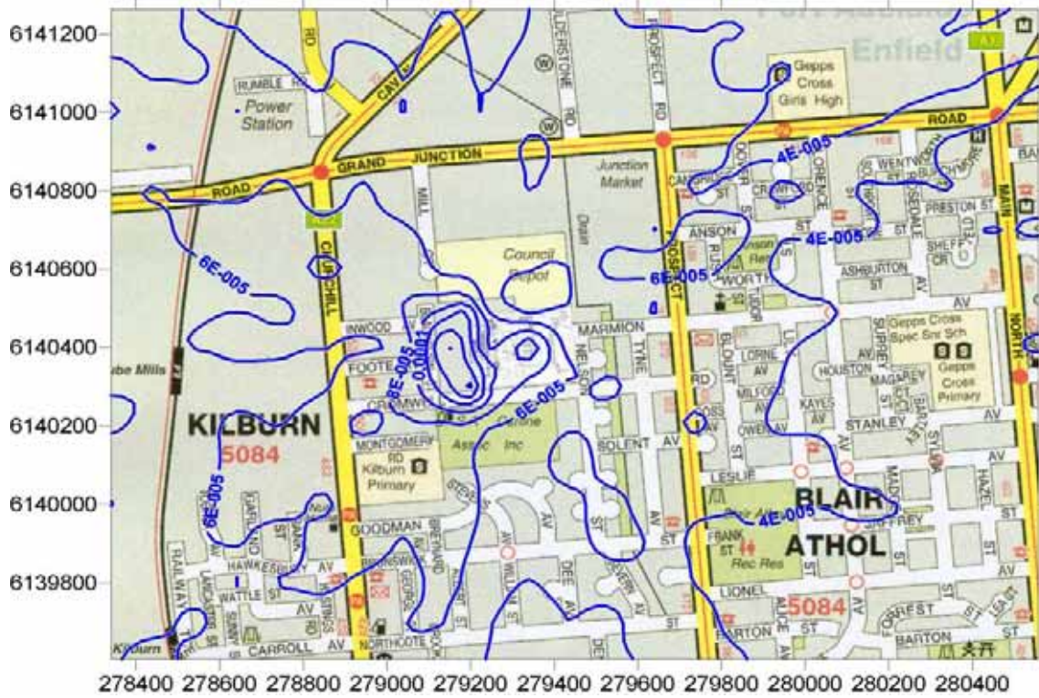
Figure 9: Predicted dioxin GLC from future (furane) operation (mg/m3). (3 minute averaging period, 100th percentile)
