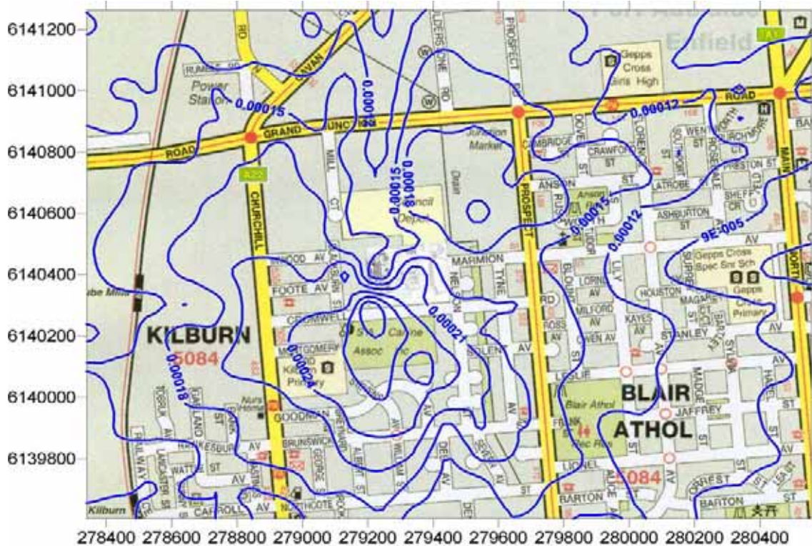
Figure 19: Predicted butyl acetate GLC from existing operation (mg/m 3 ). (3 minute averaging period, 100 th percentile)
