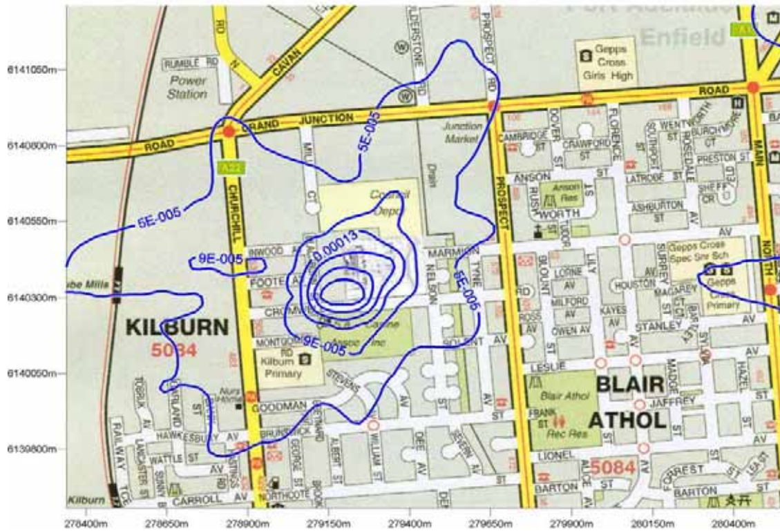
Figure 45: Predicted dimethylphenols GLC from future (furane) operation ( \text{mg}/\text{m}^3 ). (24 hour averaging period, 100 th percentile)
