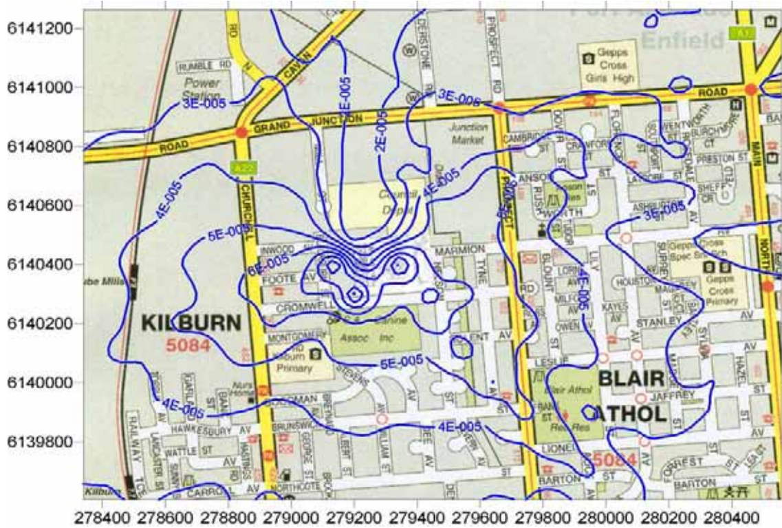
Figure 43: Predicted benzo (b) fluoranthene GLC from existing operation ( \text{mg}/\text{m}^3 ). (3 minute averaging period, 100 th percentile)
