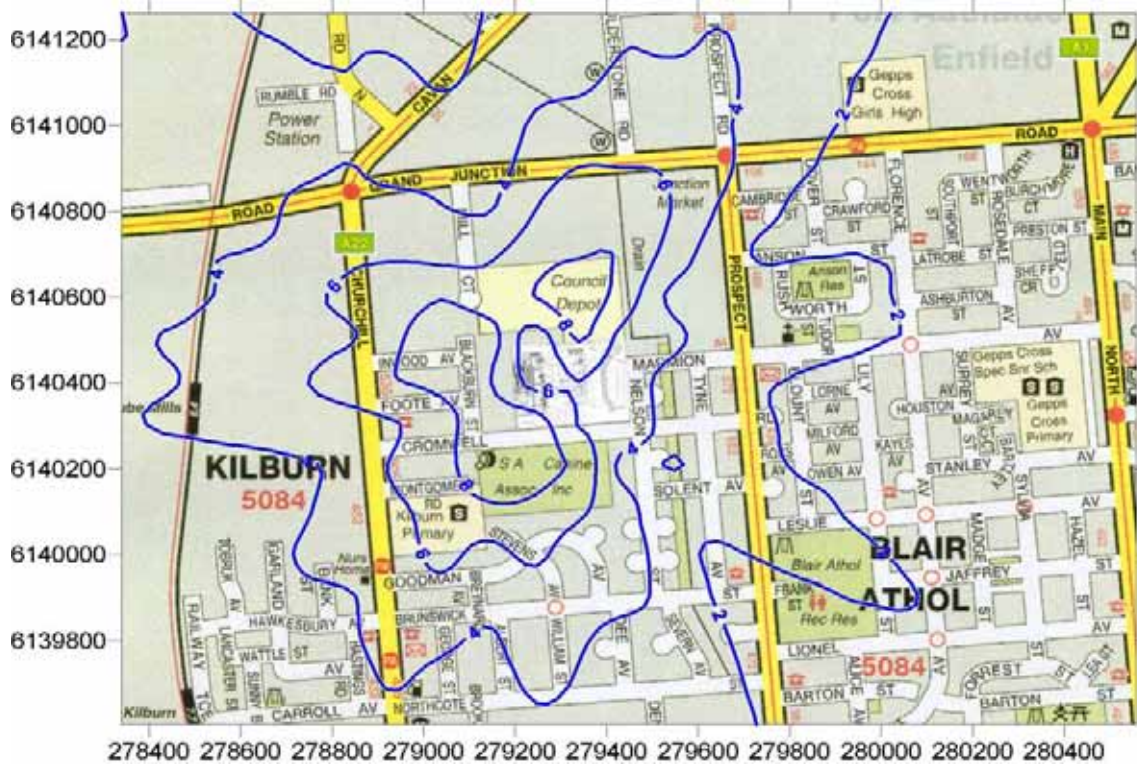
Figure 3: Predicted PM 2.5 GLC from existing operation ( \mu\text{g}/\text{m}^3 ). (24 hour averaging period, 100 th percentile)
