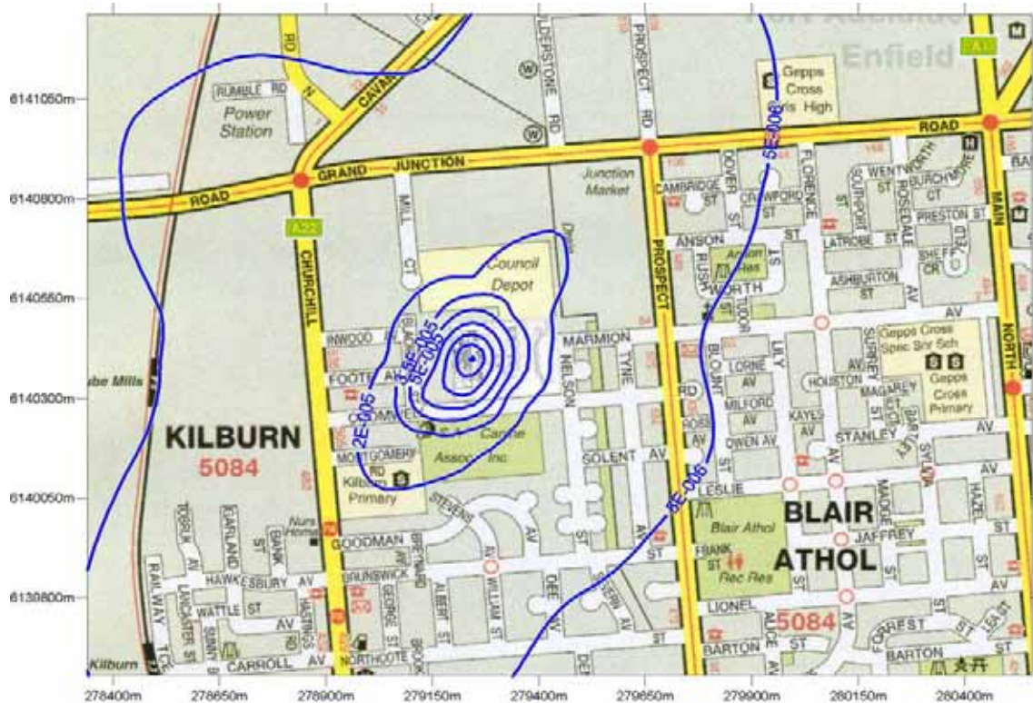
Figure 34: Predicted propanaldehyde GLC from future (furane) operation ( \mu\text{g}/\text{m}^3 ). (Annual averaging period, 100 th percentile)
