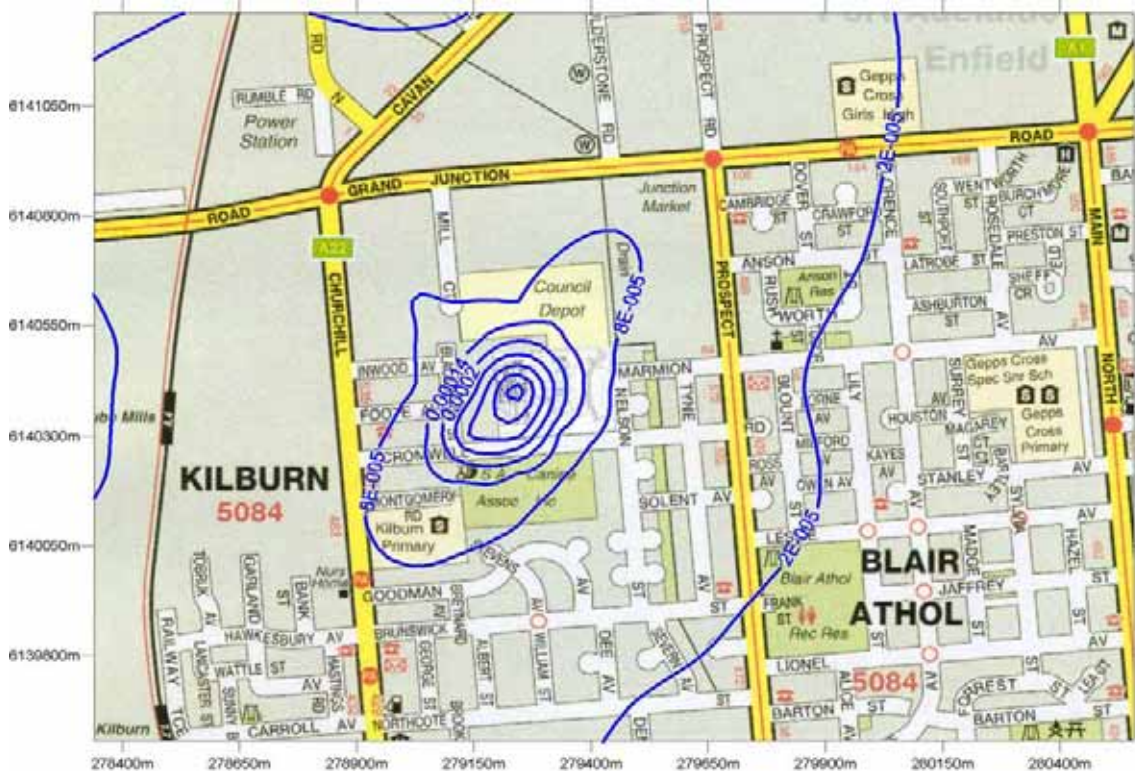
Figure 35: Predicted butanaldehyde GLC from future (furane) operation ( \text{mg}/\text{m}^3 ). (Annual averaging period, 100 th percentile)
