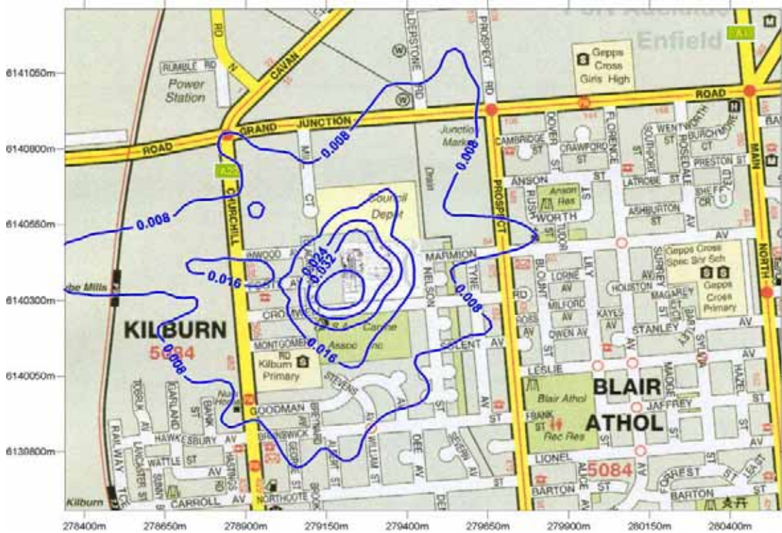
Figure 6: Predicted sulphur dioxide GLC from future (furane) operation ( \text{mg}/\text{m}^3 ). (24 hour averaging period, 100 th percentile)
