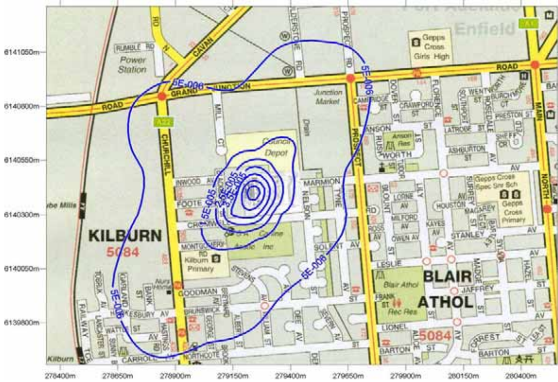
Figure 45: Predicted dimethylphenolsGLC from future (furane) operation ( \text{mg}/\text{m}^3 ). (Annual averaging period, 100 th percentile)
