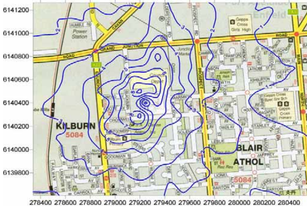
Figure 1: Predicted odour GLC from existing operation (ODU). (3 minute averaging period, 99.9 th percentile)
