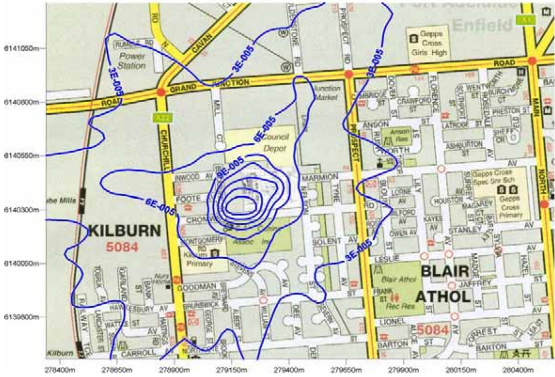
Figure 21: Predicted cyclohexanone GLC from future (furane) operation ( \text{mg}/\text{m}^3 ). (24 hour averaging period, 100 th percentile)
