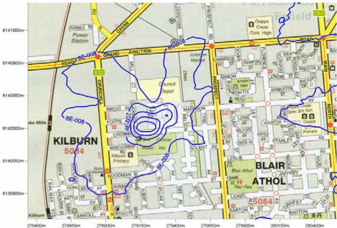
Figure 42: Predicted benzo (b) fluoranthene GLC from future (furane) operation ( \text{mg}/\text{m}^3 ). (24 hour averaging period, 100 th percentile)
