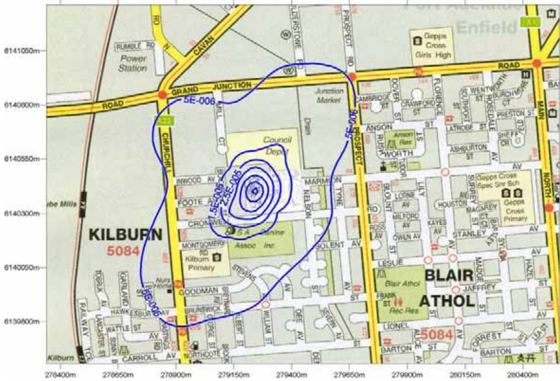
Figure 27: Predicted methylisobutylketone GLC from future (furane) operation ( \text{mg}/\text{m}^3 ). (Annual averaging period, 100 th percentile)
