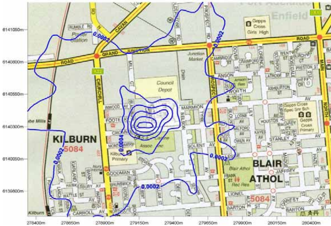
Figure 25: Predicted isopropylbenzene GLC from future (furane) operation ( \text{mg}/\text{m}^3 ). (24 hour averaging period, 100 th percentile)
