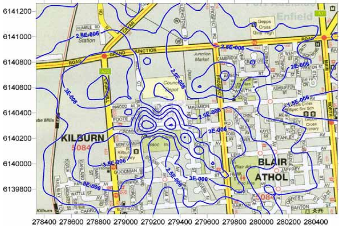
Figure 18: Predicted anthracene GLC from future (furane) operation (mg/m3). (3 minute averaging period, 100th percentile)
