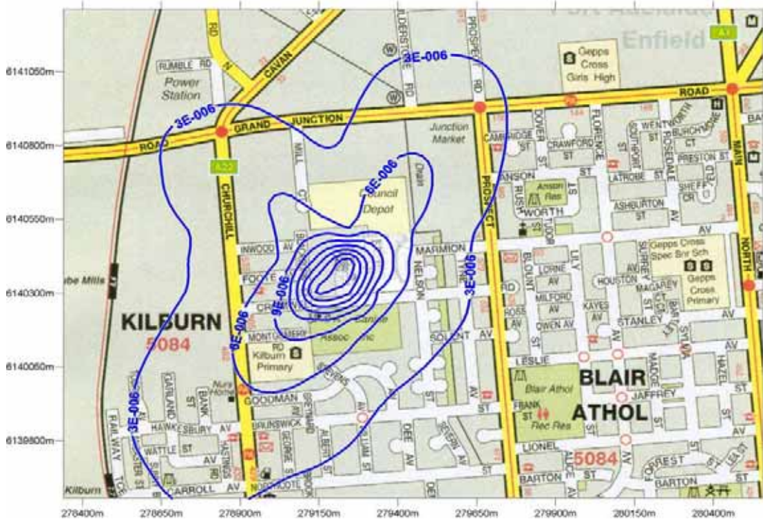
Figure 46: Predicted 1,3,5-trimethylbenzene GLC from future (furane) operation ( \text{mg}/\text{m}^3 ). (Annual averaging period, 100 th percentile)
