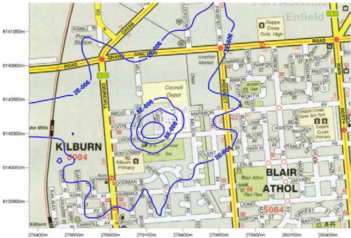
Figure 28: Predicted phenanthrene GLC from future (furane) operation ( \text{mg}/\text{m}^3 ). (24 hour averaging period, 100 th percentile)
