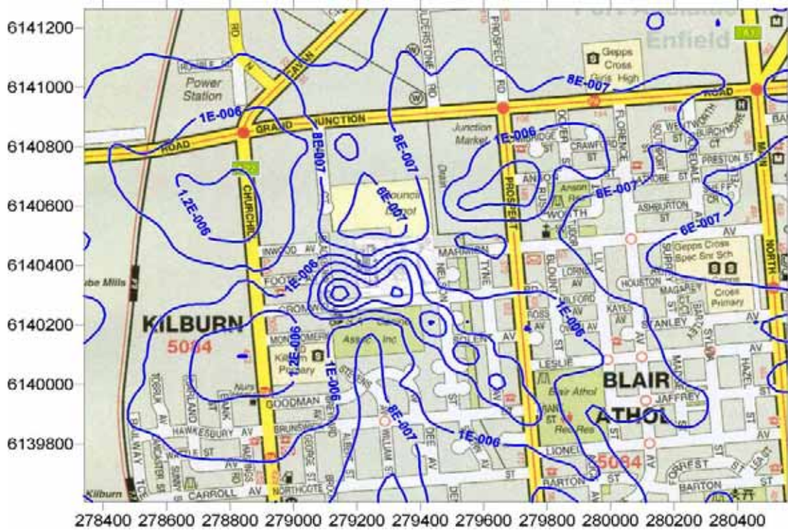
Figure 45: Predicted total fluoranthene GLC from future (furane) operation (mg/m3). (3 minute averaging period, 100th percentile)
