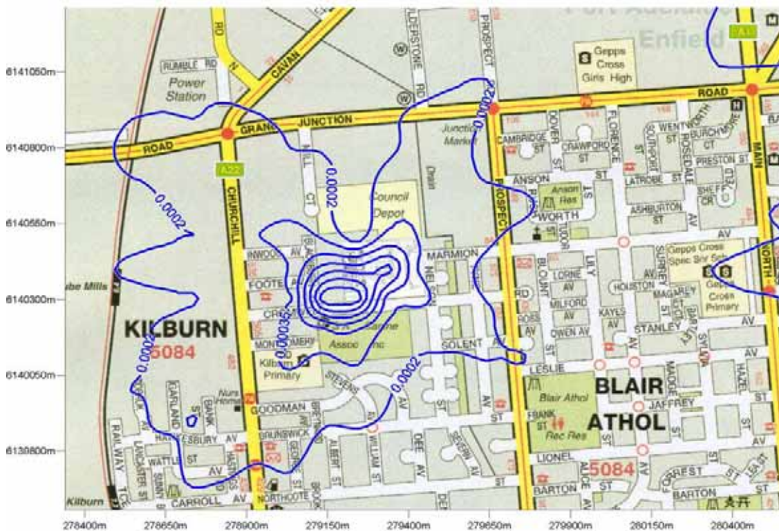
Figure 36: Predicted pentanaldehyde GLC from future (furane) operation ( \text{ng}/\text{m}^3 ). (24 hour averaging period, 100 th percentile)
