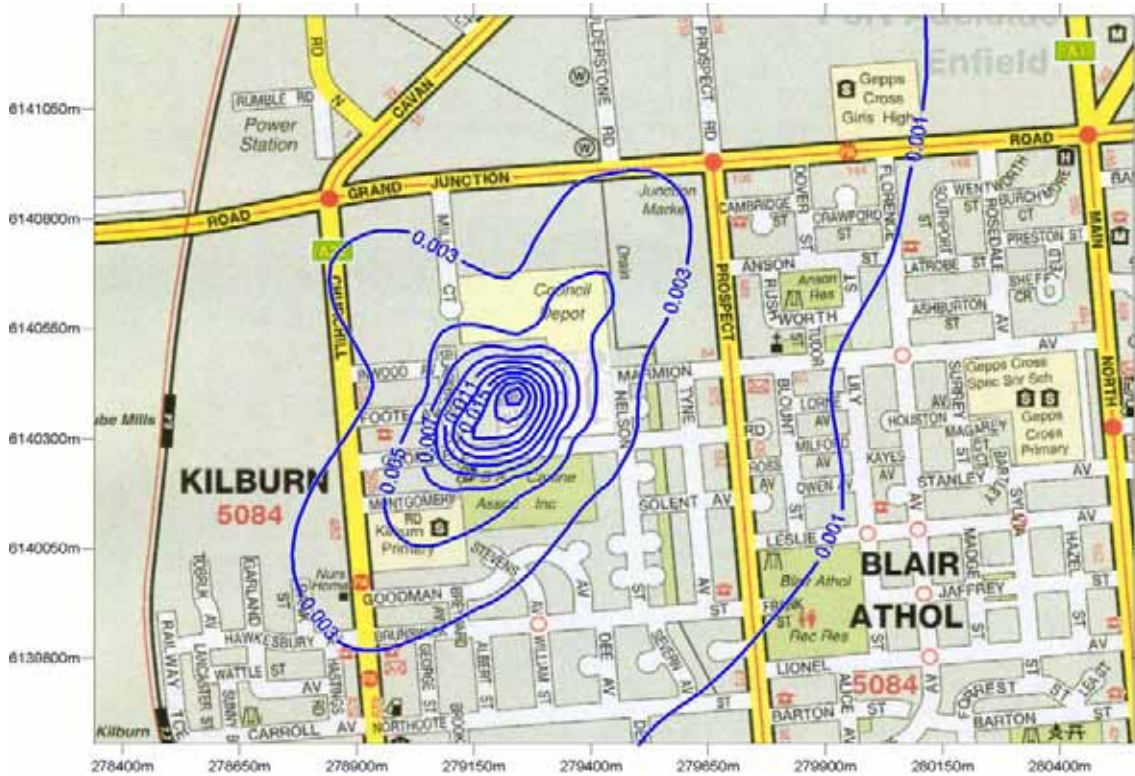
Figure 14: Predicted toluene GLC from future (furane) operation ( \text{mg}/\text{m}^3 ). (Annual averaging period, 100 th percentile)
