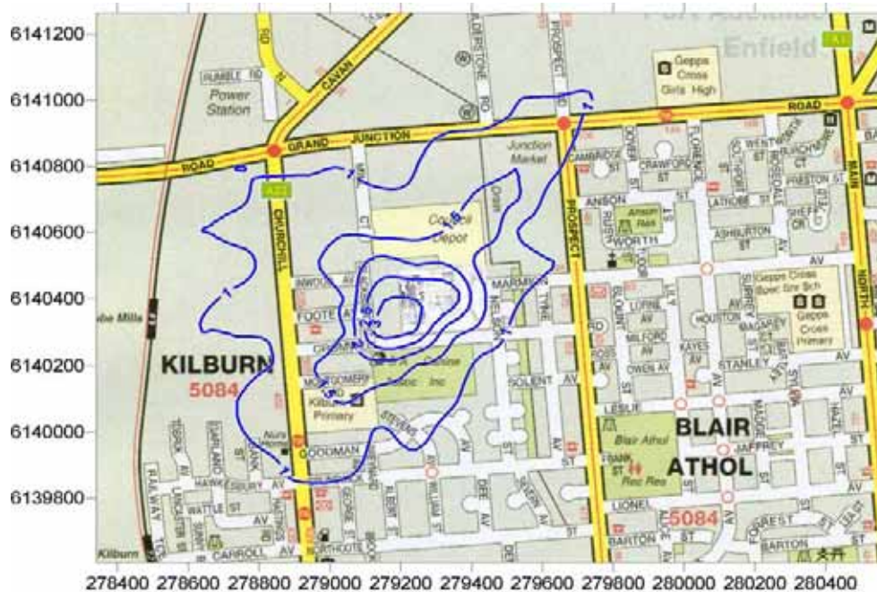
Figure 8: Predicted PM 2.5 GLC from future operation (µg/m 3 ). (24 hour averaging period, 100 th percentile)
