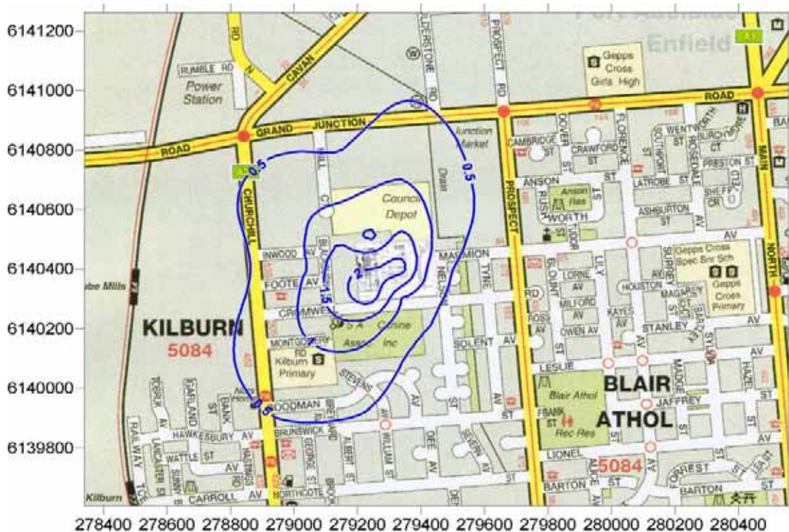
Figure 4: Predicted PM 2.5 GLC from existing operation ( \mu\text{g}/\text{m}^3 ). (Annual averaging period, 100 th percentile)
