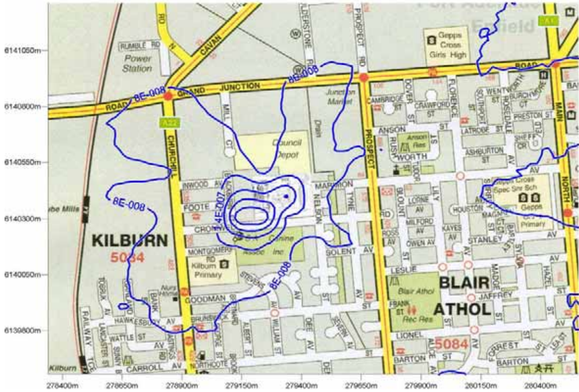
Figure 41: Predicted benz (a) anthracene GLC from future (furane) operation ( \text{mg}/\text{m}^3 ). (24 hour averaging period, 100 th percentile)
