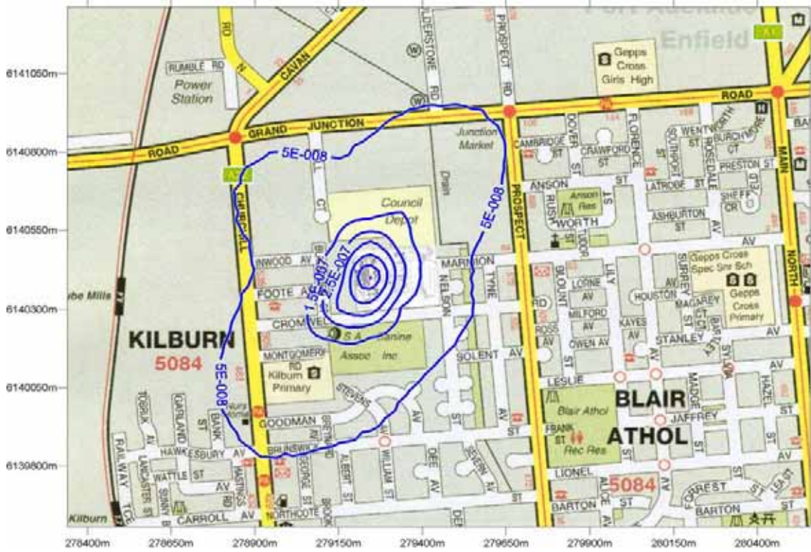
Figure 29: Predicted pyrene GLC from future (furane) operation ( \text{mg}/\text{m}^3 ). (Annual averaging period, 100 th percentile)
