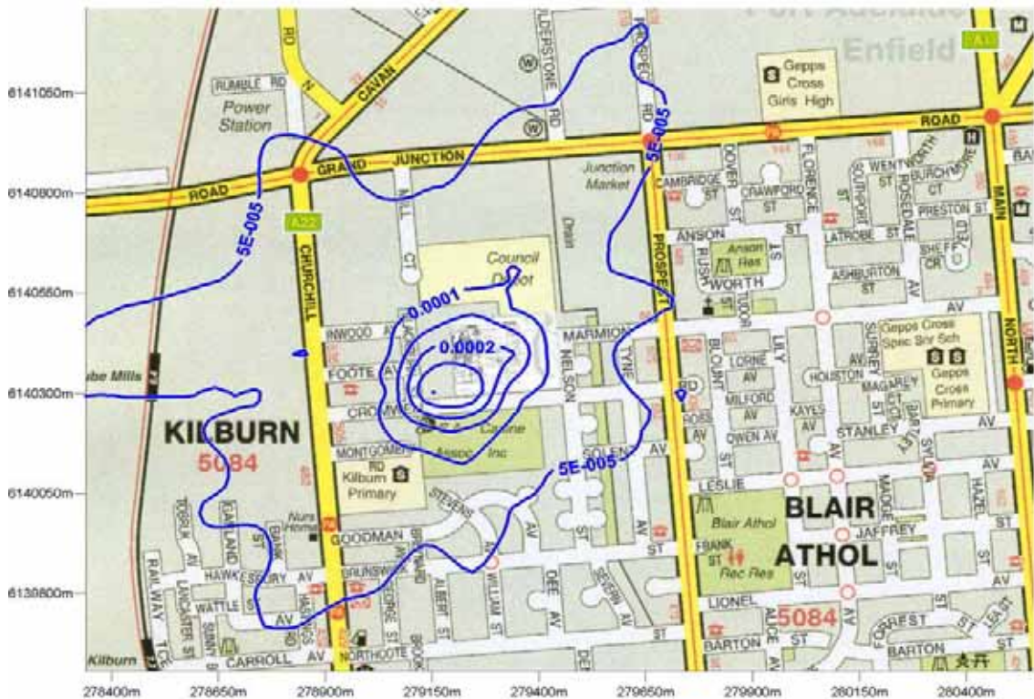
Figure 30: Predicted styrene GLC from future (furane) operation ( \text{mg}/\text{m}^3 ). (24 hour averaging period, 100 th percentile)
