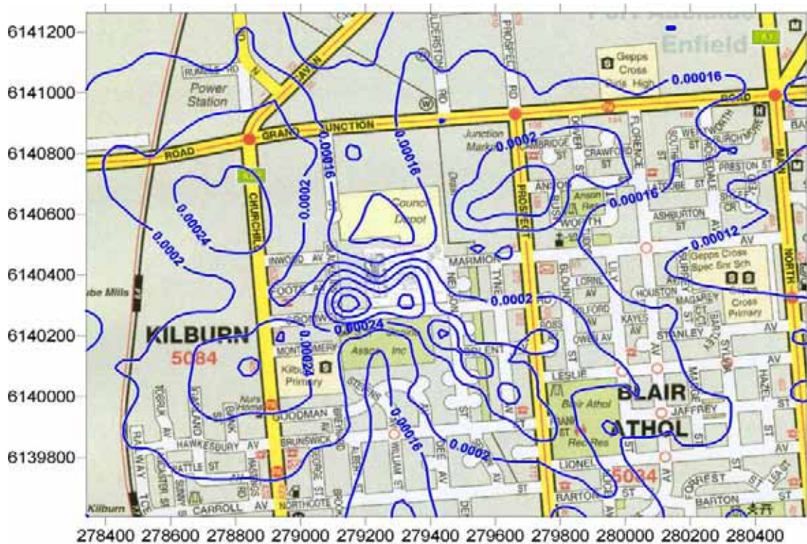
Figure 48: Predicted 1,3,5-trimethylbenzene GLC from future (furane) operation (mg/m3). (3 minute averaging period, 100th percentile)
