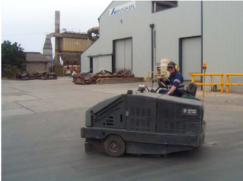
Figure 19: Vacuum street sweeper used to remove dust from roads and hard stand areas around the site.
