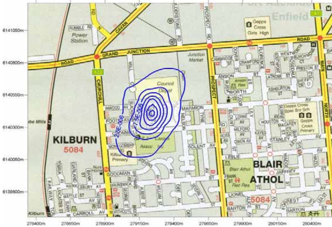
Figure 15: Predicted acrolein GLC from future (furane) operation ( \text{mg}/\text{m}^3 ). (Annual averaging period, 100 th percentile)
