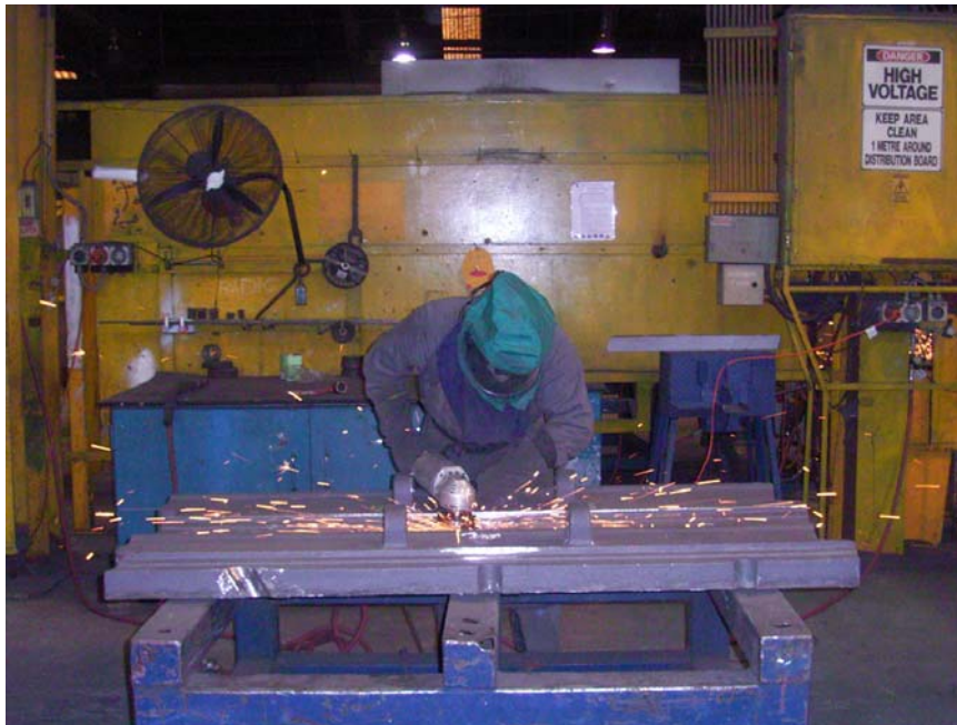
Figure 10: Casting are cleaned and dressed in the Aftercast area
