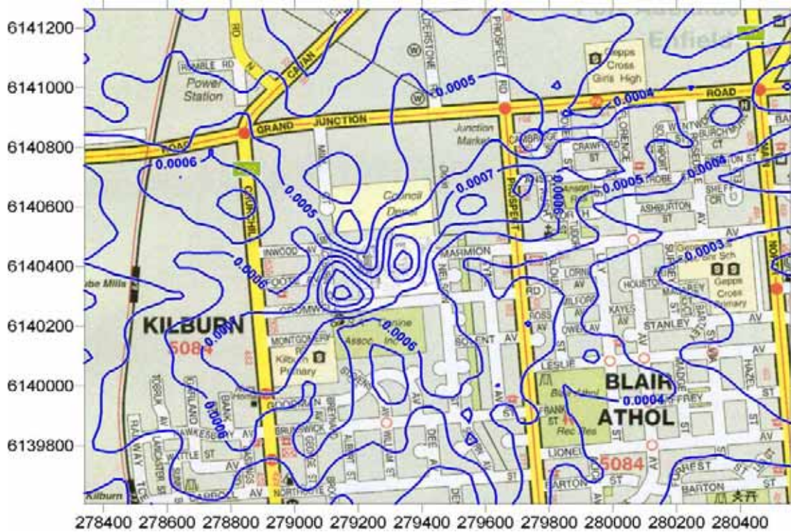
Figure 39: Predicted benzaldehyde GLC from future (furane) operation (ug/m3). (3 minute averaging period, 100th percentile)
