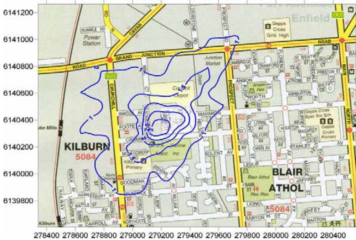
Figure 6: Predicted PM2.5 GLC from future (furane) operation (ug/m3). (24 hour averaging period, 100th percentile)
