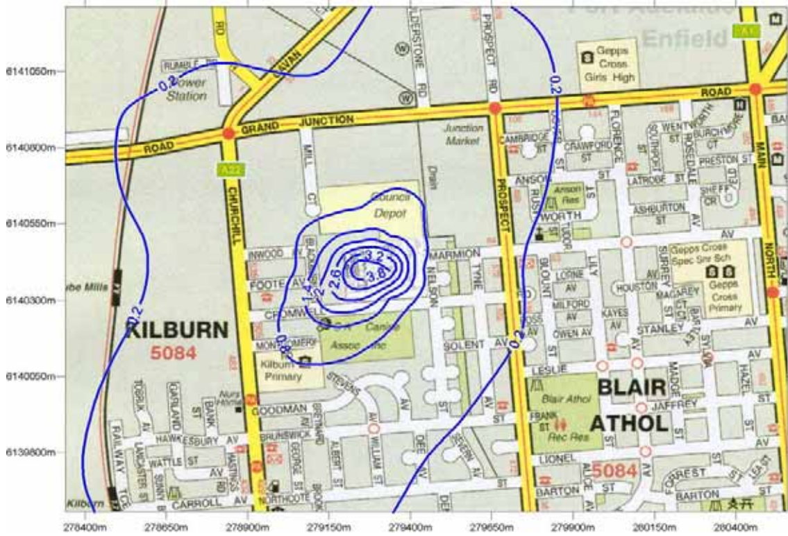
Figure 3: Predicted PM10 GLC from future (furane) operation ( \mu\text{g}/\text{m}^3 ). (Annual averaging period, 100 th percentile)
