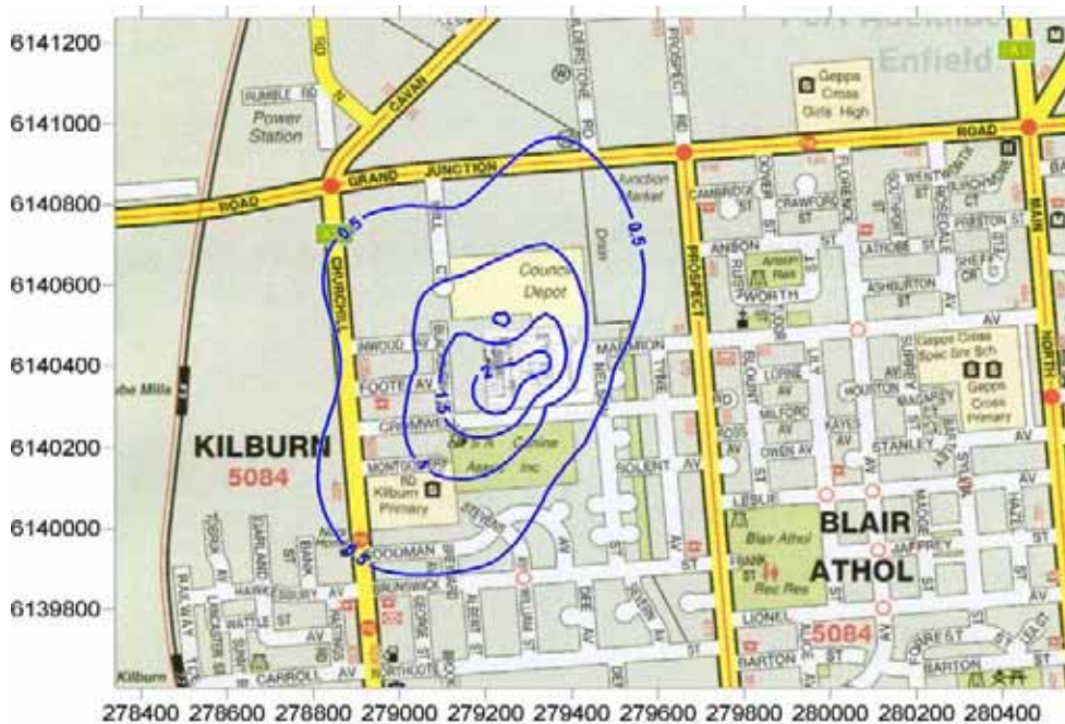
Figure 9: Predicted PM 2.5 GLC from existing operation (µg/m 3 ). (Annual averaging period, 100 th percentile)
