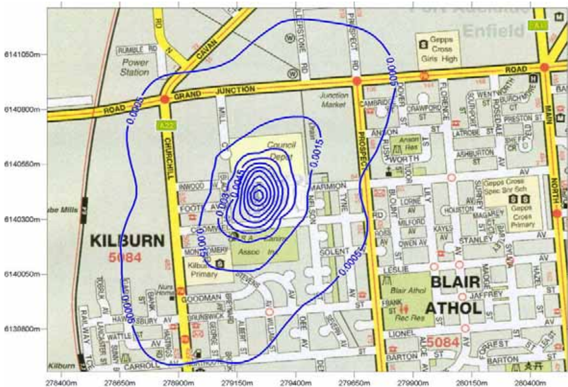
Figure 6: Predicted sulphur dioxide GLC from future (furane) operation ( \text{mg}/\text{m}^3 ). (Annual averaging period, 100 th percentile)
