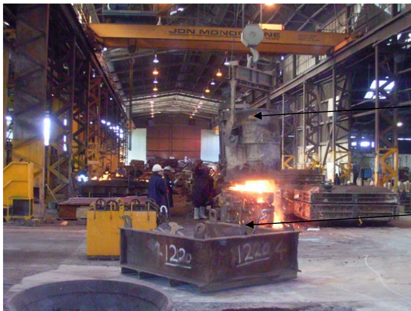
Figure 7: Molten metal is poured from the ladle into individual sand moulds.
