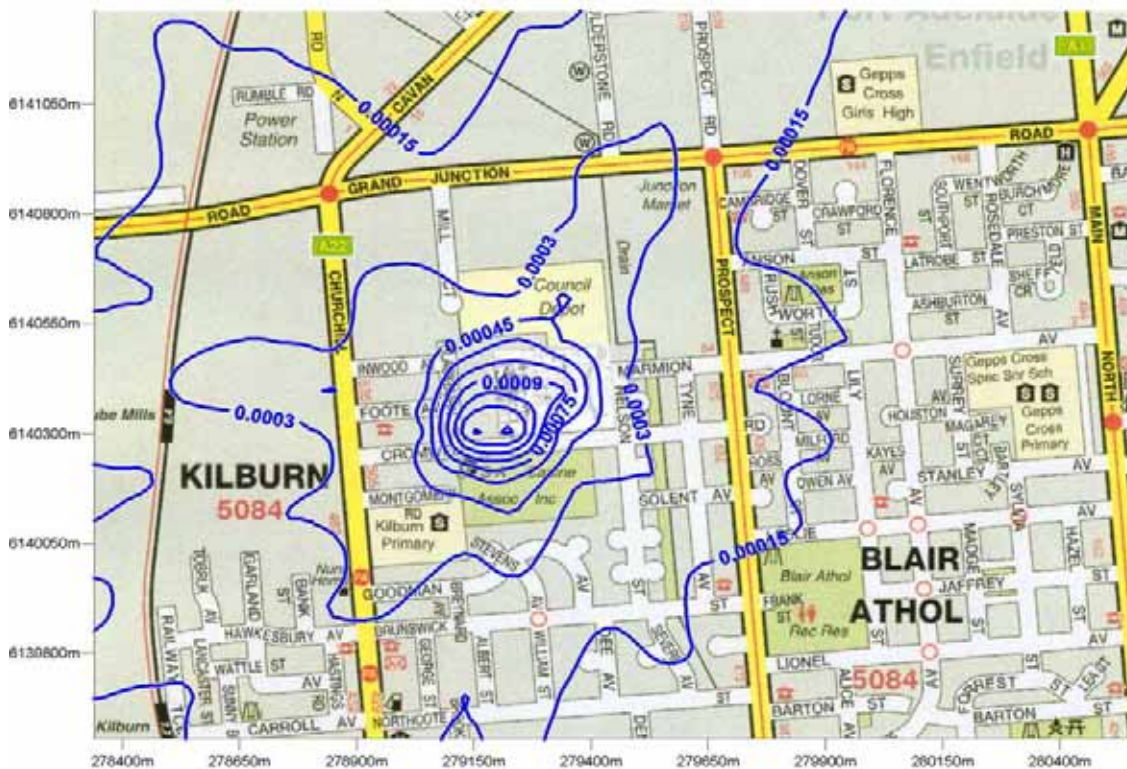
Figure 26: Predicted methylethylketone GLC from future (furane) operation ( \text{mg}/\text{m}^3 ). (24 hour averaging period, 100 th percentile)
