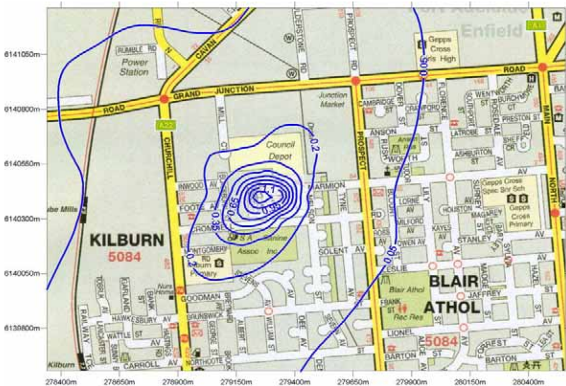
Figure 4: Predicted PM2.5 GLC from future (furane) operation ( \mu\text{g}/\text{m}^3 ). (Annual averaging period, 100 th percentile)
