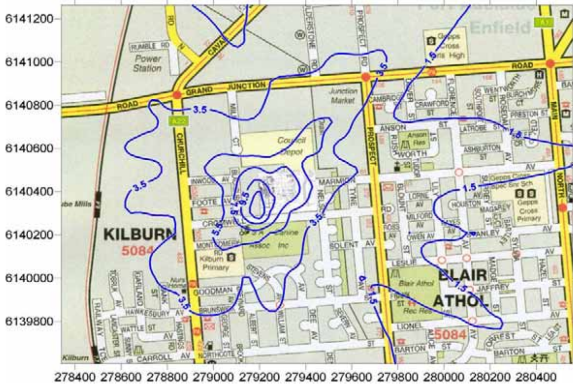
Figure 5: Predicted PM10 GLC from future (furane) operation (ug/m3). (24 hour averaging period, 100th percentile)
