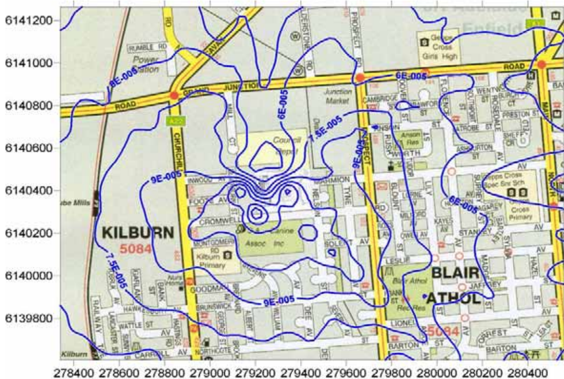
Figure 29: Predicted phenanthrene GLC from existing operation ( \text{mg}/\text{m}^3 ). (3 minute averaging period, 100 th percentile)
