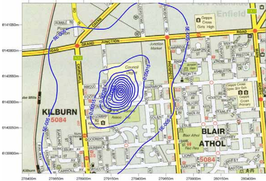
Figure 2: Predicted hydrogen sulphide GLC from future (furane) operation ( \text{mg}/\text{m}^3 ). (Annual averaging period, 100 th percentile)
