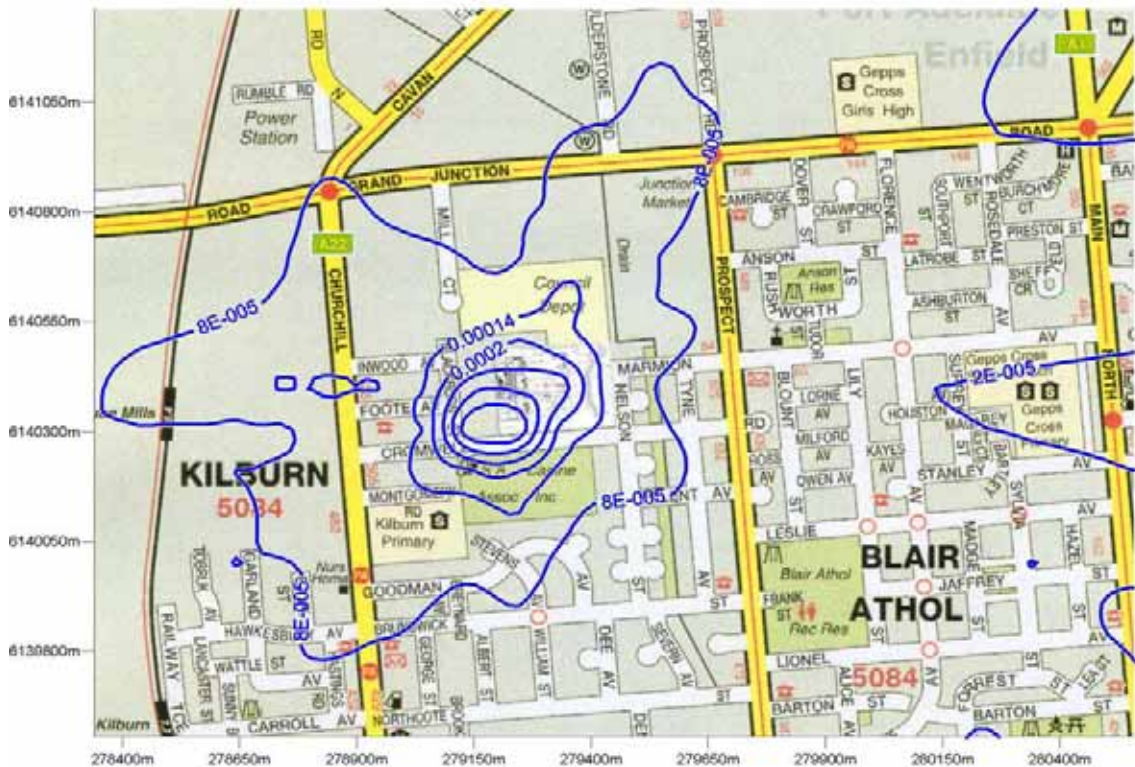
Figure 34: Predicted propanaldehyde GLC from future (furane) operation ( \mu\text{g}/\text{m}^3 ). (24 hour averaging period, 100 th percentile)
