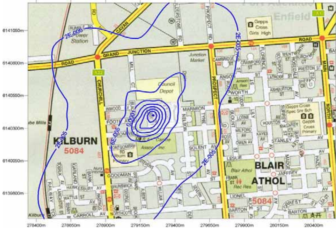
Figure 25: Predicted isopropylbenzene GLC from future (furane) operation ( \text{mg}/\text{m}^3 ). (Annual averaging period, 100 th percentile)
