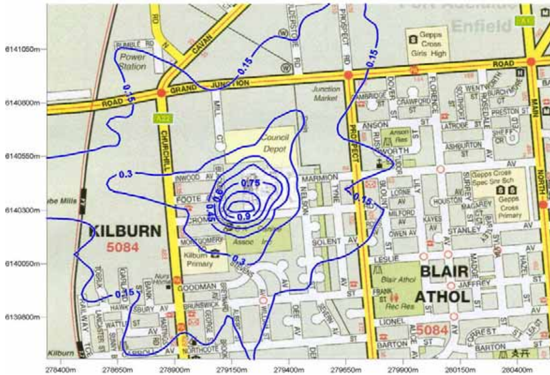
Figure 19: Predicted carbon monoxide GLC from future (furane) operation ( \text{mg}/\text{m}^3 ). (24 hour averaging period, 100 th percentile)
