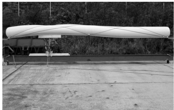
Fig. 4 Strong pneumatic structures with Tensairity: Tensairity demonstration bridge with 8 m span and 3.5 tons maximal load (left) and an ultimate load test of a Tensairity beam (right).
