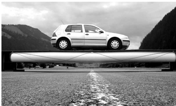
Fig. 4 Strong pneumatic structures with Tensairity: Tensairity demonstration bridge with 8 m span and 3.5 tons maximal load (left) and an ultimate load test of a Tensairity beam (right).
