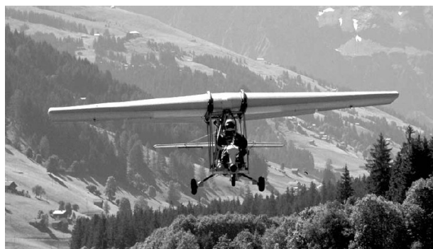
Fig. 2. New pneumatic structures: The inflated airplane Stingray (left) and the inflated wing Pneuwing (right).
