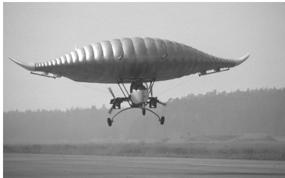
Fig. 2. New pneumatic structures: The inflated airplane Stingray (left) and the inflated wing Pneuwing (right).
