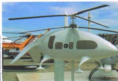
Mockup of the EADS SHARC with its contra-rotating coaxial twin-rotor system. Its payload was to have included a conformal-array radar.
