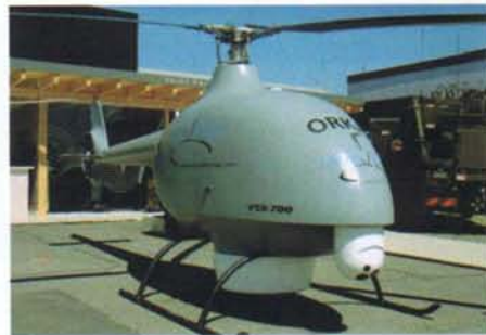
EADS’ Orka-1200 proposal has the capacity to carry both an air-surface radar and a gyro-stabilised electro-optical/infrared sensor ball.
