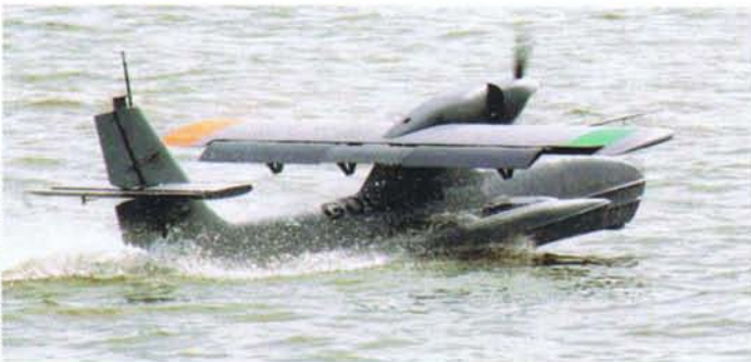
The Warrior Gull 36 is claimed to be able to take off and land dependably in Sea State 5.5, thanks to its wave-piercing hull form and sophisticated wave-sensing flight control system.
