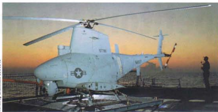
Northrop Grumman's MQ-8B Fire Scout is undergoing flight tests from the frigate USS McInerney prior to trials with the USN's new Littoral Combat Ships.
