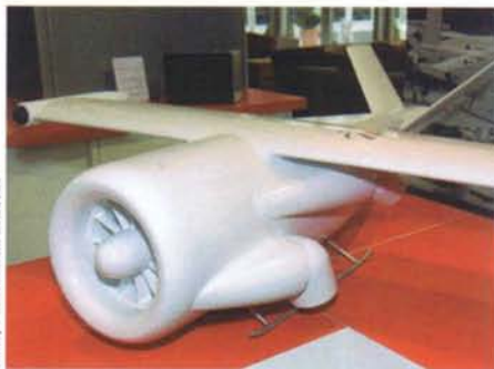
Model of the Selex Damsel fly vectored-thrust UAV with its wing-tip sensor pods.
