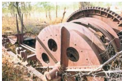
63. Winding drums at the Pump Shaft.
