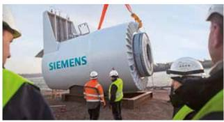
Siemens 3.0 MW direct drive wind turbines offer innovation through the consistent implementation of a highly efficient generator concept. With half the parts of conventional geared turbines and much less than half the number of moving parts, the direct drive wind turbines are easy to maintain and extremely reliable. The compact design allows for cost-effective transportation on standard vehicles in most markets.
