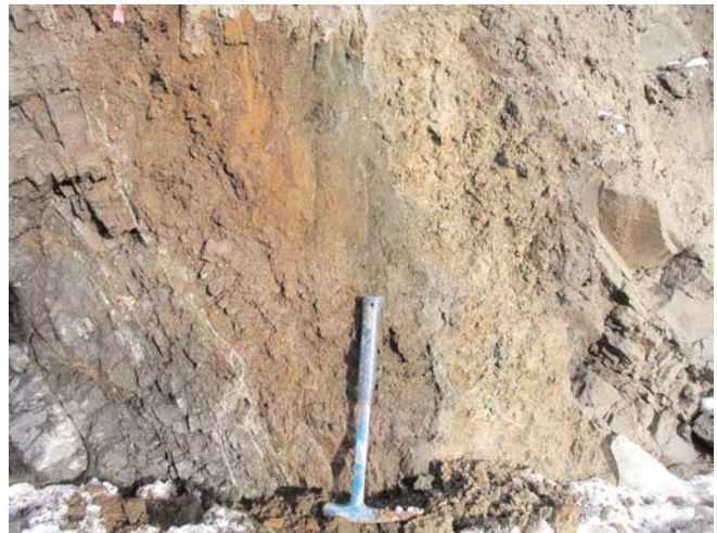
Figure 6. Contact of the A154 South kimberlite (left) and wallrock (right).
