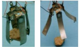
FIGURE 1: 4-finger EAP gripper lifting a rock.
