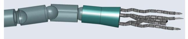
FIGURE 7: A graphic view of an octopus-configured catheter for surgical applications.
