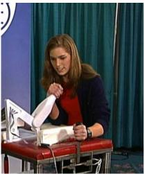
2. The Swiss arm (Figure 4) was able to resist for 4-seconds before losing. This arm was driven by the dielectric elastomer EAP type using multi-layered scrolled actuators that were organized in 4 groups. A photo of one of the group lifting two 5-gallon water containers (about 20-kg) is shown in Figure 5. These actuators were operated similar to
