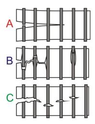
Each fiber breakage is reflected in a peak in the "force-displacement" diagram. The critical force for the first fiber is larger than for the others.
