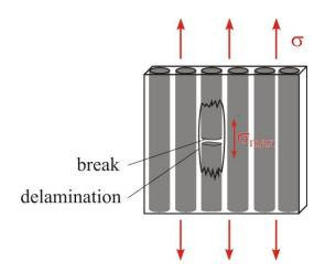
There is shear stress concentration at the bond surface between components. Stress concentration in laminate materials is higher than in isotropic materials. Thus, the strength of a notched composite specimen is rather high.
