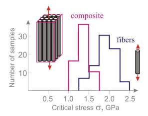
For constant average strength and higher scatter, there is a higher probability that microcracks in the weakest fibers are surrounded by strong fibers. The ultimate strength of such composites is usually high.
