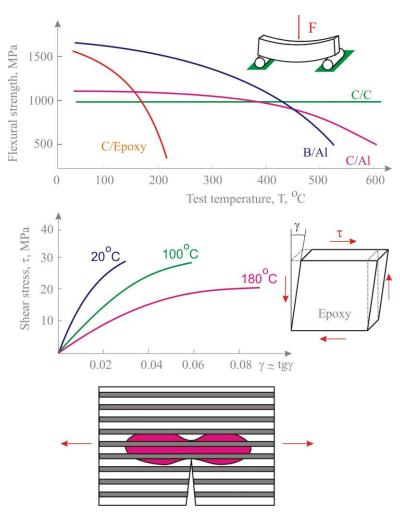
The creep rate increases as nominal stress increases. The ductility of the matrix contributes significantly to the creep effect. Reinforcement by strong and rigid fibers along the direction of the force leads to higher creep strength.
