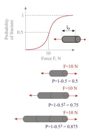
If the probability of fracture of a fiber with length  $l_{\circ}$  is 0.5, then the probability of failure of a longer fiber is higher. Fibers with longer length have lower strength. Composite series-parallel structures do not decrease the strength to zero due to strength redundancy of parallel elements.
