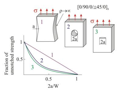
Tensile strength decreases "faster" than shear strength in the presence of voids and cracks in multilayer composites.
