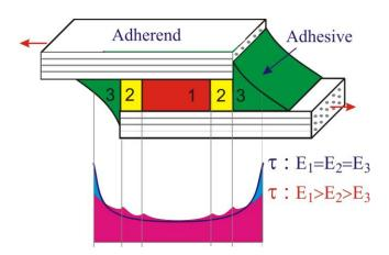
Stress concentration is smaller for a "smooth" transition from one structural element (adherent) to another.
