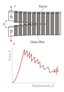
Unidirectional composites have a high crack resistance if the maximum tensile stress acts along the fibers. Tension in the transverse direction demonstrates a crack resistance that is lower than the same parameter for a ductile matrix.
