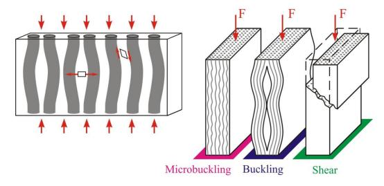
A honeycomb composite structure has high flexural strength. The mechanisms of stability loss under compression depends on many factors, such as adhesive quality, size of honeycomb, fiber filament, and other factors.
