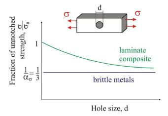
Cracks perpendicular to the applied load are more dangerous than a hole with the same maximum size.
