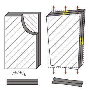
Tangential stress in the pressure vessel is twice as large as radial stress. The stress ratio defines the optimal angle of two-directional lay-up: 55°.
