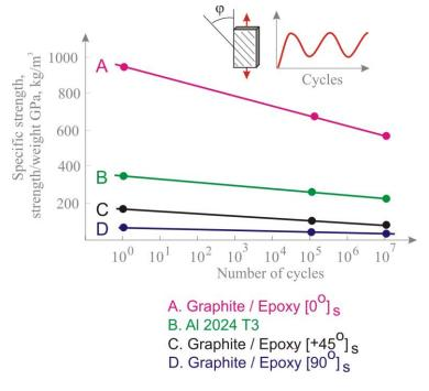
The use of composite materials decreases the weight of a passenger airplane by 20 - 40%. Use of composite materials decreases the cost of many engineering structures. An increase in fiber content does not excessively raise the cost of the composite.
