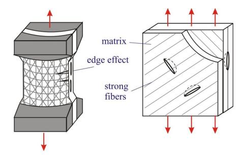
Holes and cracks decrease the tensile strength of composites. Composite materials are less "sensitive" to small defects.
