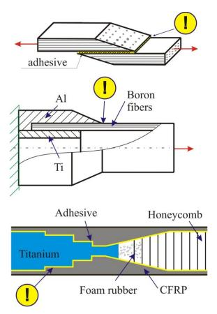
Stress concentration is higher in a more rigid material. Proper laminar orientation can decrease the stress concentration.
