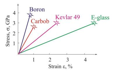
Fibers differ from other structural materials due to a larger scatter in experimental data.
