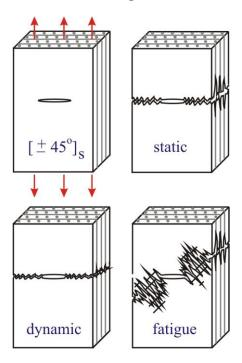
Voids in the matrix decrease the strength of unidirectional composites. The effect of strength decrease is highest for transverse tension and shear, and lower for tension along the fibers.
