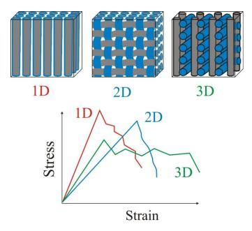
The modulus of elasticity of a composite material depends on the component's parameters, fiber content, and structure of the composite.
