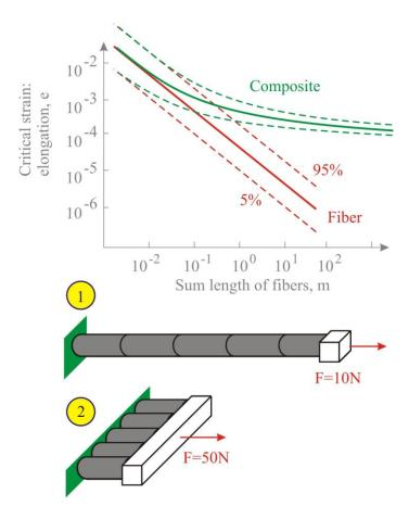
The probability of failure of a series structure composed of similar elements (fibers) is higher than that for a parallel structure.
