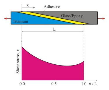
The joint's bond surface must be sufficiently larger than its cross-sectional area. The joint can be reinforced by fabric fibers.
