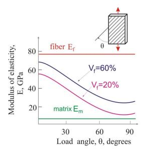
Stiffness of a fabric depends upon the load angle. An angle of 45° corresponds to minimum rigidity. Stiffness of straight fibers is higher than that for curved fibers.
