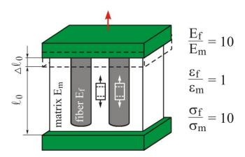
The stress pattern in a composite beam demonstrates higher stress in rigid components and in external layers. Local delamination and voids have a small effect on the flexural stiffness of the composite beam.
