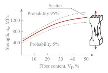
Higher average strengths correspond to higher scatter in experimental data. This rule is valid for fibers and composite materials.
