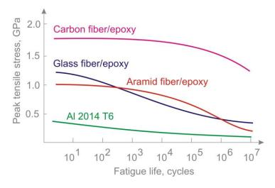
At the first stage of cycling, the "weak" fibers are broken. The composite does not fail at this stage due to redundancy of strength. Delamination and microstructural bond damage occurs
