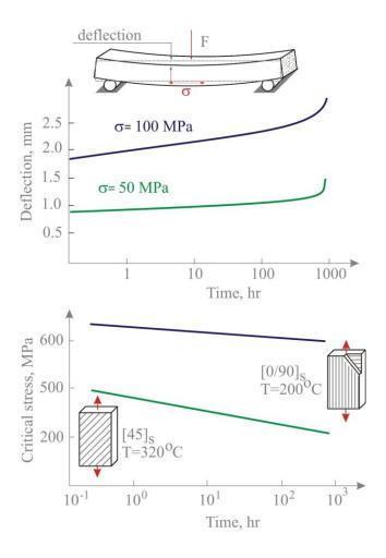
Glass fiber becomes more brittle and weaker at the "explosive" deformation rate - small values of the parameter.
