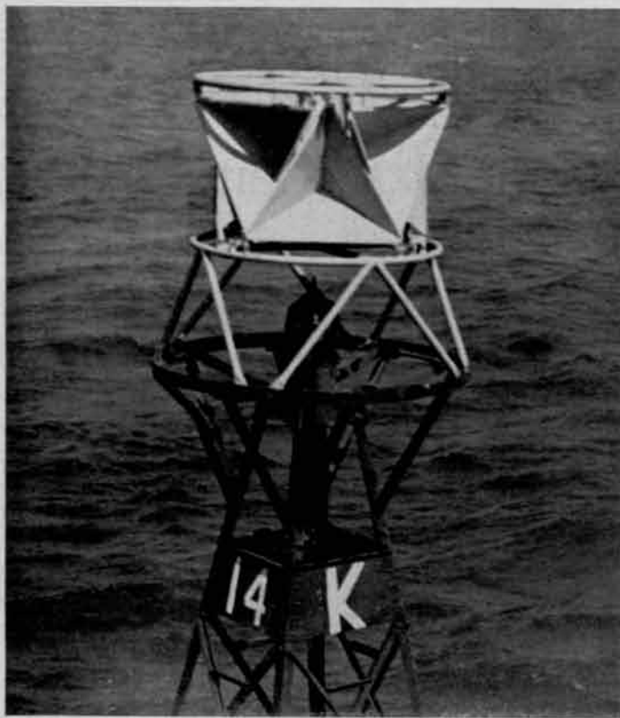
Figure 2. Basic type Trihedral reflector used here by U. S. Coast Guard to mark a buoy.
