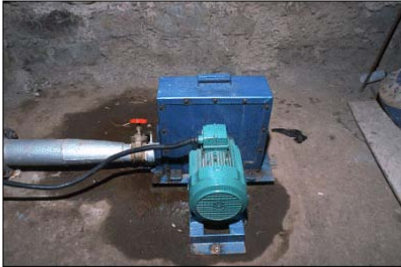
A pico generator using a regular motor (Source: www.tve.org )
