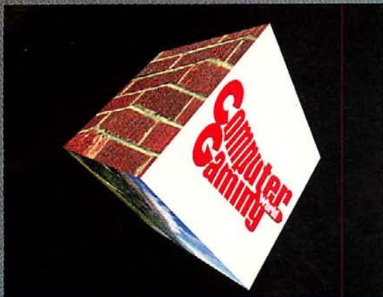
Perspective Correction prevents texture maps from "warping" when they're moved to different positions.
