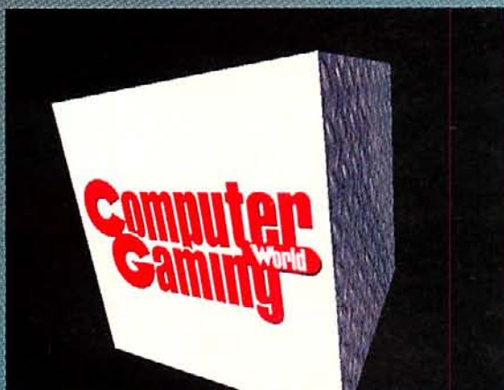
Anti-aliasing prevents the "stair-step" effect noticeable on the edges of the cube.
