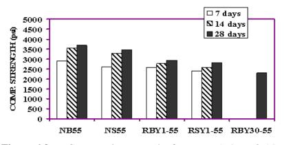
**Figure 6.3** Compressive strength of concrete (w/cm =0.55).
