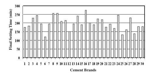
Figure 4.2 Final setting time of cement brands.
