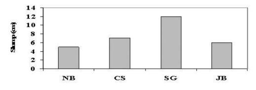
**Figure 5.1** Workability of concrete made with different aggregates (w/cm =0.55).
