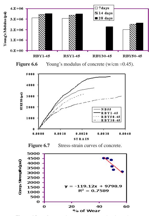
Figure 6.8 Compressive strength versus abrasion value.
