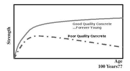
Figure 6.9 Schematic of strength of concrete versus time.
