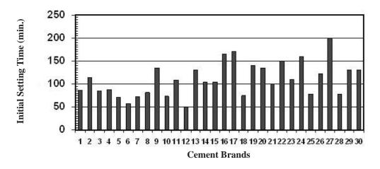
**Figure 4.1** Initial setting time of cement brands.
