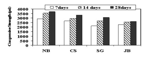
**Figure 5.2** Compressive strength of concrete made with different aggregates.
