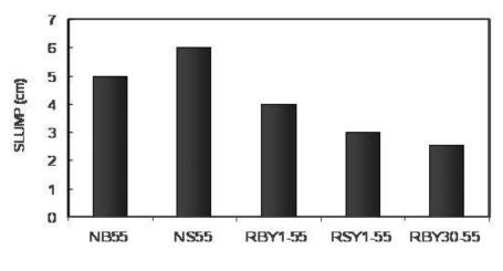
**Figure 6.1** Workability of concrete (w/cm =0.55).
