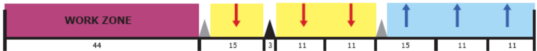
Stage 1: Five lanes to the right of the median barrier, one lane to the left.
