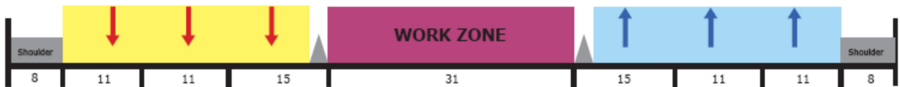
Stage 3: Work zone is in the median between temporary barriers
