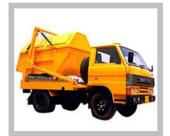
load dumper placers (for transporting 4.5 cubic meter secondary containers) are proposed to be used for transportation of MSW.
