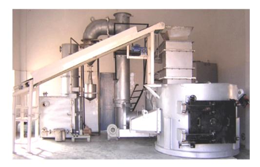
The design of the incinerator is categorized into two stages based on the combustion process. The first stage would be primary combustion chamber wherein the dead carcass would be further processed by drying, physical separation of water & carbon dioxide, decomposition of all compounds and combustibles and burning the carbon in a controlled environment.
