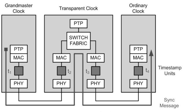
Sync Correction Field =  $t_3 - t_2$
