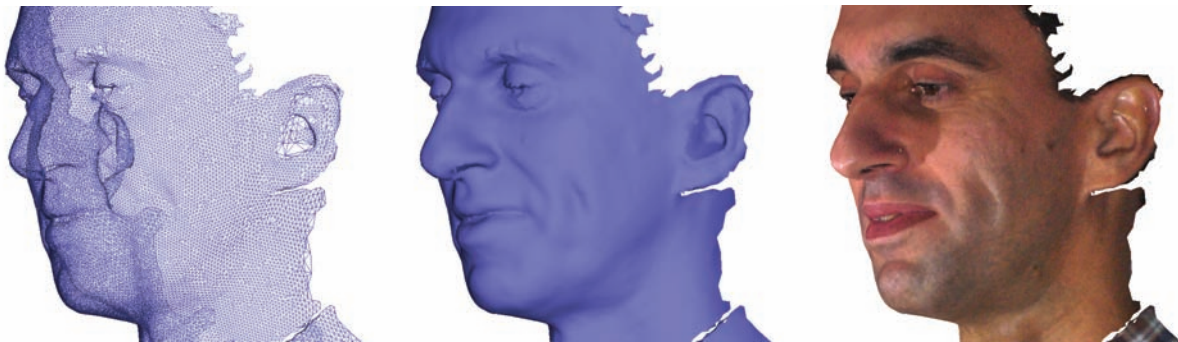
Figure 17. 3D photograph imported as a mesh, rendered as a wireframe model, a smooth surface and a textured surface.
