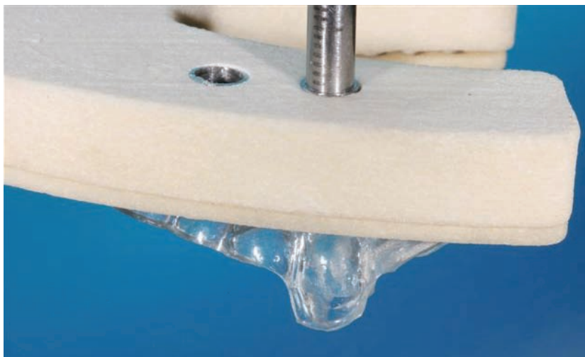
Figure 6. Real volume over the Flatguide™, with the sleeves and the calibrated rod
