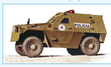
The ALIGATOR 4x4 police modification preserves the primary concept of the driving system, including the self-supporting vehicle hull. The transporter is specially adjusted to the police needs. The six crew PCM version is recognizable by the addition of four firing ports in the windshield, the vehicle sides, and the rear door and can be fitted with front mounted barricade-remover, flashing beacons, public address system and tear-gas grenade discharges.
