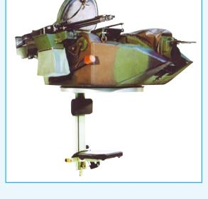
Recently developed modification has roof-mounted a one-man armoured observation cupola The cupola is fitted with a day/night thermal camera, day periscope, externally mounted 7.62 mm machine gun and smoke grenade launchers.
