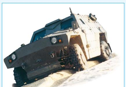
The driver has a roof-mounted periscope for forward observation located above his seat. The commander and driver are each provided with a large bulletproof window to their front and a door in the side that opens forwards.
