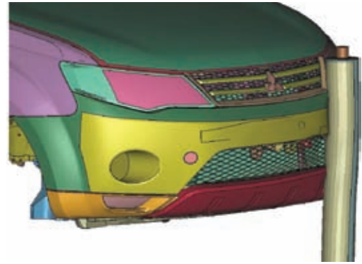
図6 歩行者保護CAE解析状況(バンパー部) CAE analysis for pedestrian protection (bumper)
