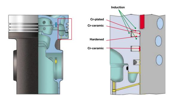
engine, the pressure balance above and below each ring is crucial. Experience has shown that this effect is most likely achieved with a three-ring pack. Finally, it is well known that most frictional losses in a reciprocating combustion engine originate from the rings. Thus a three-ring pack is the obvious choice in this respect, too. The piston ring package and ring grooves are optimized for long lifetime by special wear-resistant coating and groove treatment.
