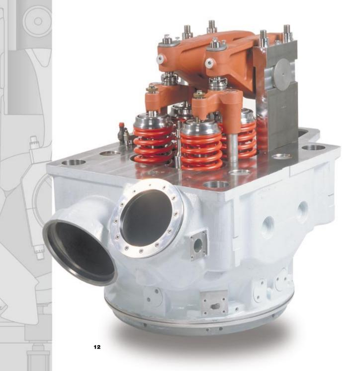
The cylinder head design is based on the four-screw concept developed by Wärtsilä and used for almost 20 years. A four-screw cylinder head design also provides all the freedom needed for designing inlet and exhaust ports with a minimum of flow losses. The port design has been optimized using computational fluid dynamics (CFD) analysis in combination with full-scale flow measurements.
