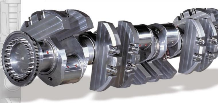
The latest advances in combustion development require a crank gear which can operate reliably at high cylinder pressures. The crankshaft must be robust and the specific bearing loads kept at an acceptable level. This is achieved by careful optimization of crankthrow dimensions and fillets. The specific bearing loads are conservative and the cylinder spacing, which is important for the overall length of the engine, is minimized.
