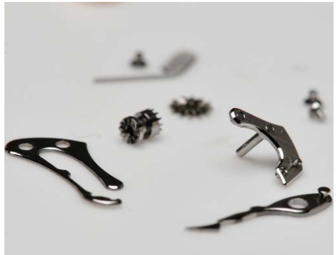
Parts of the setting mechanism.
