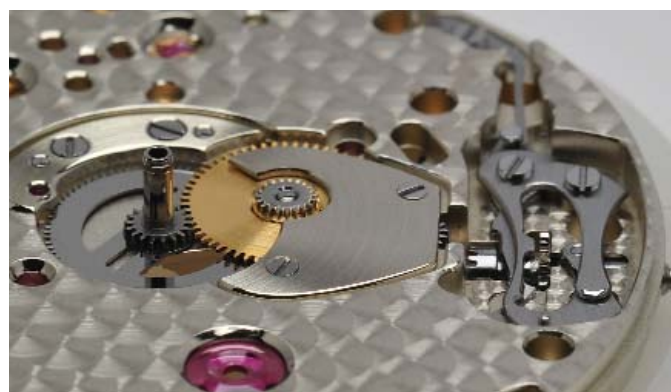
Dial side of the SM-2 showing detail of the setting mechanism.
