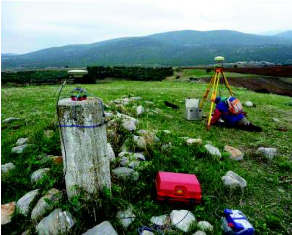
Figure 4.2 Outline of the GPS Base station (on the pillar) together with the location of the Gravity Base station.
