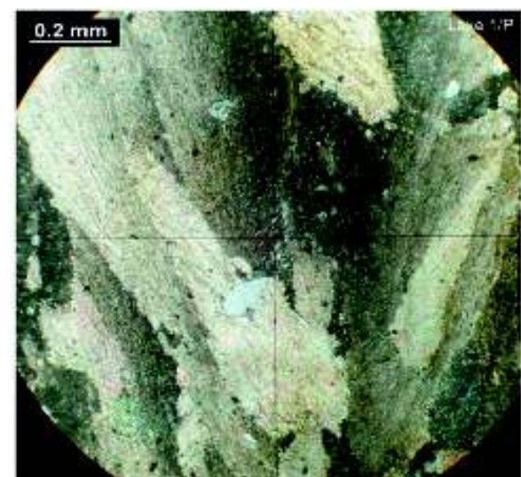
F Detail of crystall growth of spinifex calcite including small quartz clasts
