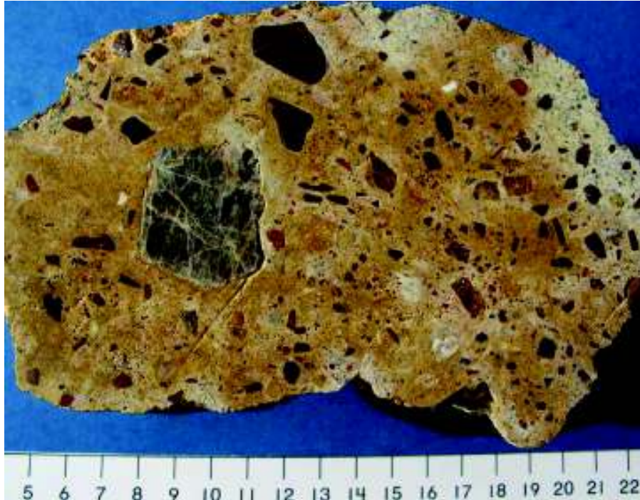
Figure 14 Polygenic impact breccia type A, lake 2. Broken fragments of quartz and reddish to brownish radiolarian cherts ( \text{SiO}_2 ) are distributed chaotically in a fine-grained calcite matrix with abundant feathery spinifex textures (Plate IVb).
