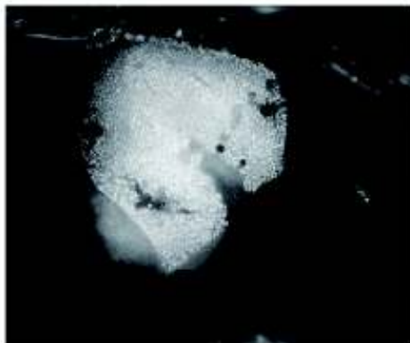
High-temperature effects; melted (decomposed) zircon into a granular aggregate of the mineral baddeleyite ( ZrO_2 ) (small bright dots) and silica glass (grey); Aouelloul Crater (Mauritania). Decomposition at experimental temperatures of 1750^\circ C .
