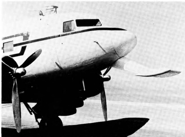
Pod-mounted infra-red radiometer on UCSD's DC-3 aircraft is used to measure solar energy released from oceans.
