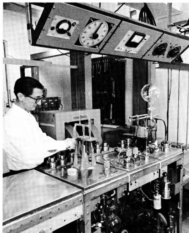
The Scripps-developed Omegatron, a sensitive analytical gas mass spectrometer, is applied to oceanographic research.
