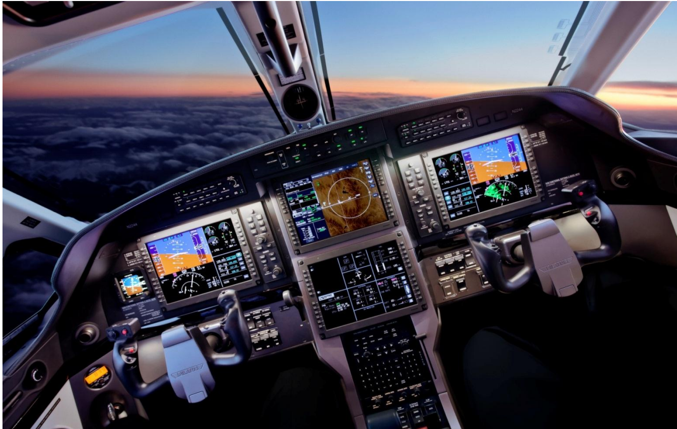
The Honeywell Primus Apex Avionics Suite in the Pilatus PC-12 NG
