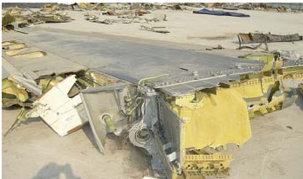
[Figure 21] Left Horizontal Stabilizer
