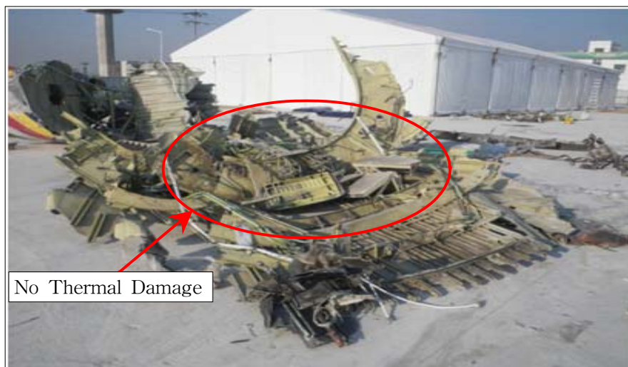
[Figure 30] Wreckage behind Aft Pressure Bulkhead
