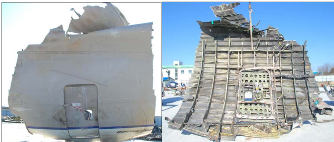
[Figure 23] Exterior and Interior Side of the L5 Door
