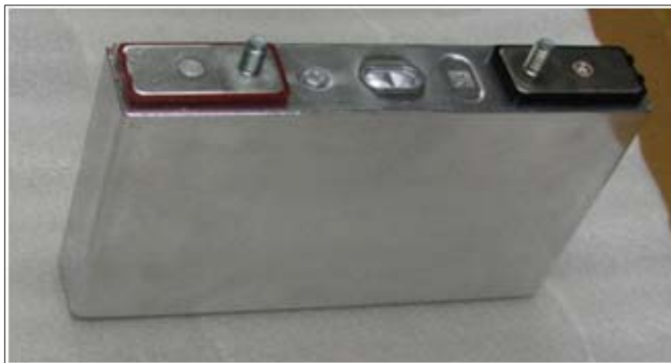
[Figure 41] 1-Cell Battery
