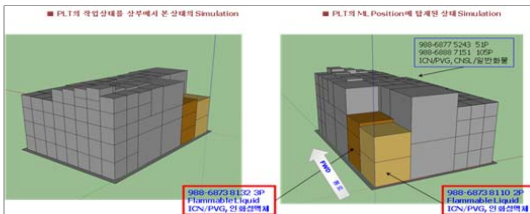
[Figure 49] Reconstruction of Loading of ML Pallet (PMC11978OZ)
