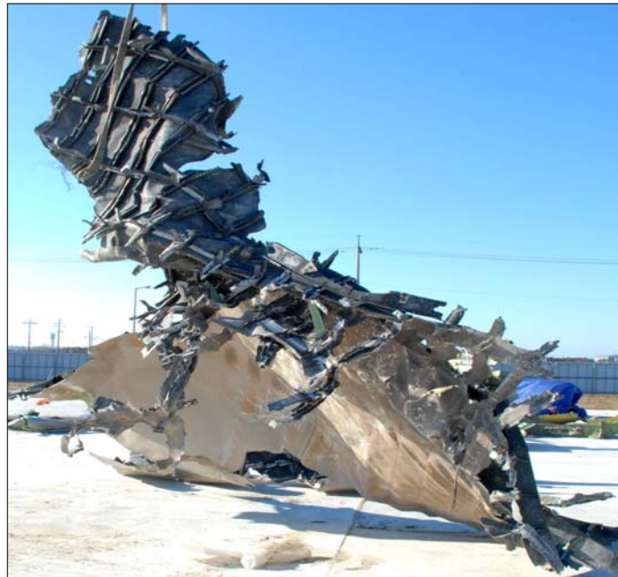
[Figure 24] Fire Damage to the Skin
