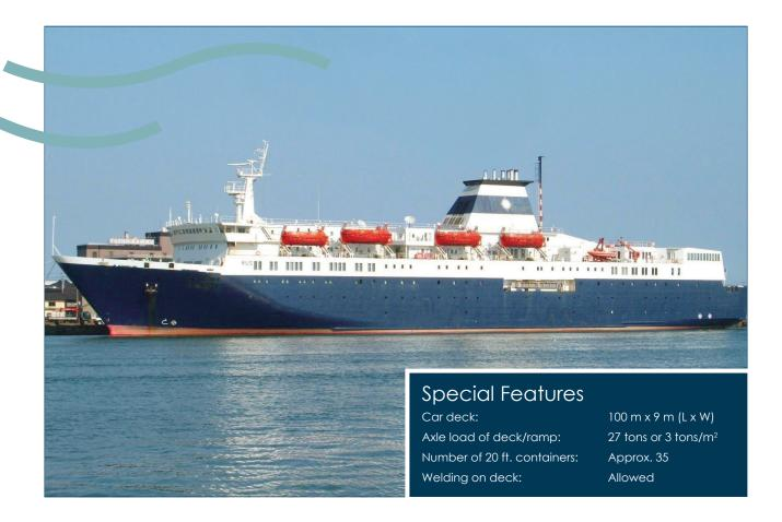
Built: 1986 8325432 IMO: 139.55 mtr Length overall: Breadth: 21.00 mtr Max draft: 5.80 mtr GT: 12,798 mts NT: 4,653 17 knots Max speed:
