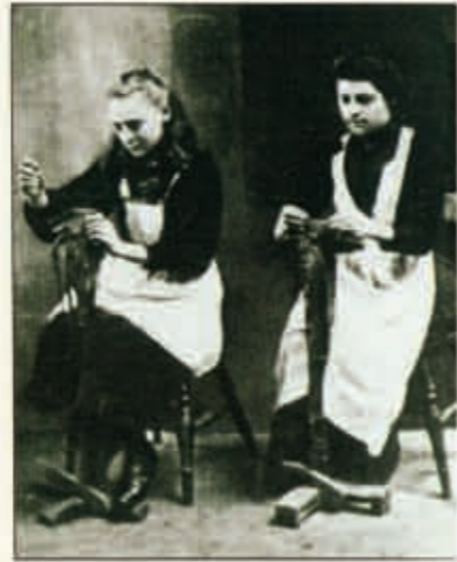
Using a "donkey" frame to hold the glove while it is being sewn. Dents factory, circa 1900.
