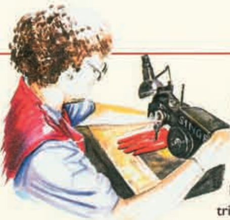
Sewing the "points" to the back of the glove. Only the hand and eye of the skilled machinist ensures accuracy. Dents factory, Warminster, England.
