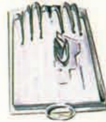
Gloving Punch, as used for over 200 years.
