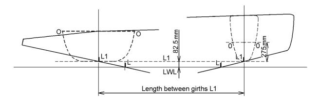
23.2.5 Immersion marks I, in accordance with the diagram, on both sides of the yacht shall be midway between the girth stations with the bottom corners just touching the waterline. When measured in fresh water additional I marks are to be placed according to its different specific gravity.
