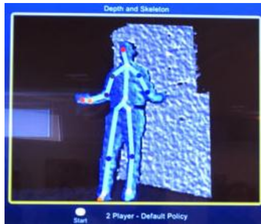
Figure 5. A laboratory view of a graphical representation of skeletal tracking data.
