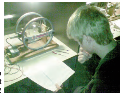
Jay Cooper studying the instructions for measurement of e/m using Helmholtz Coils and a cathode-ray tube.
