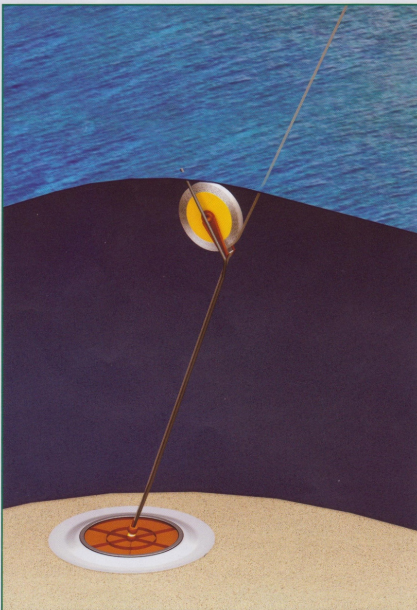
Figure 2. Parts of the proposed system: the suction pad with knuckle joint, tension cable with suction hose, and floating reel with ribbon cable
