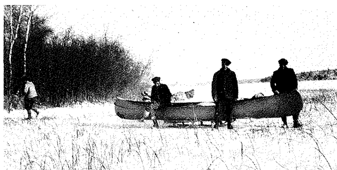
An all-purpose canoe that could be pulled over the ice on runners and when open water had to be crossed the sled was removed. (H. Ennis 1928)
