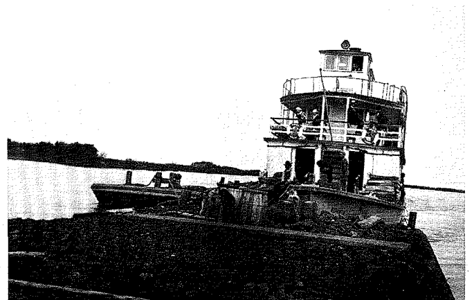
The barges were pushed by boat (S. S. Nipawin) to The Pas. The ore was then loaded into boxcars and shipped to the Smelter at Trail, B.C. Approximately 26,000 tons of ore was shipped from 1917 to 1920. (Manitoba Archives)
