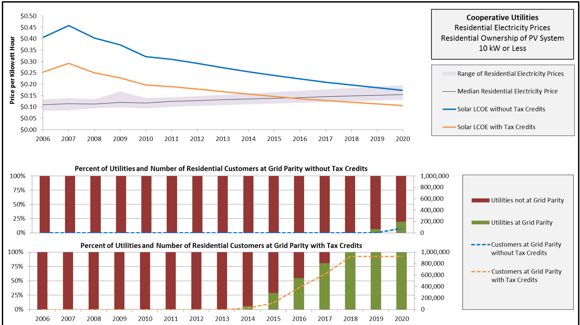
Figure 5. Scenario 1 - LCOE of Solar PV Systems 10 kW or Less and Cooperative Residential Electricity Prices.
