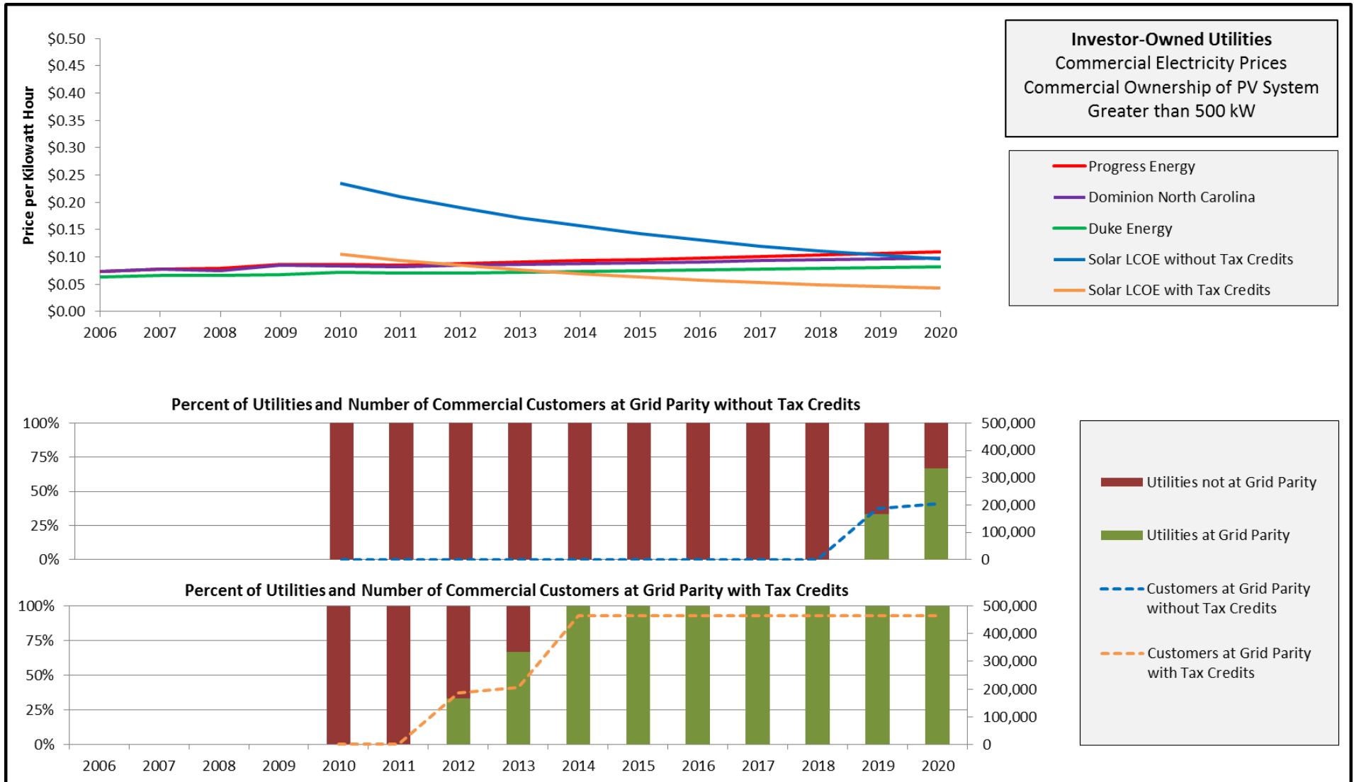
Figure 13. Scenario 9 - LCOE of Solar PV Systems Greater than 500 kW and Investor-Owned Commercial Electricity Prices.
