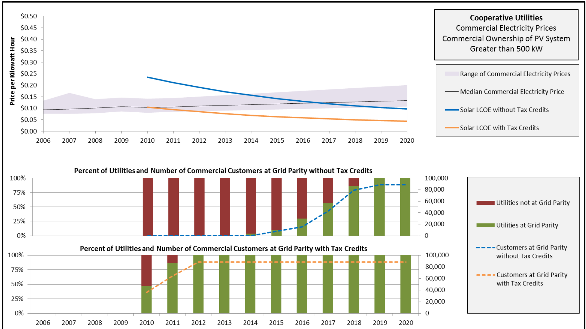
Figure 11. Scenario 7 - LCOE of Solar PV Systems Greater than 500 kW and Cooperative Commercial Electricity Prices.
