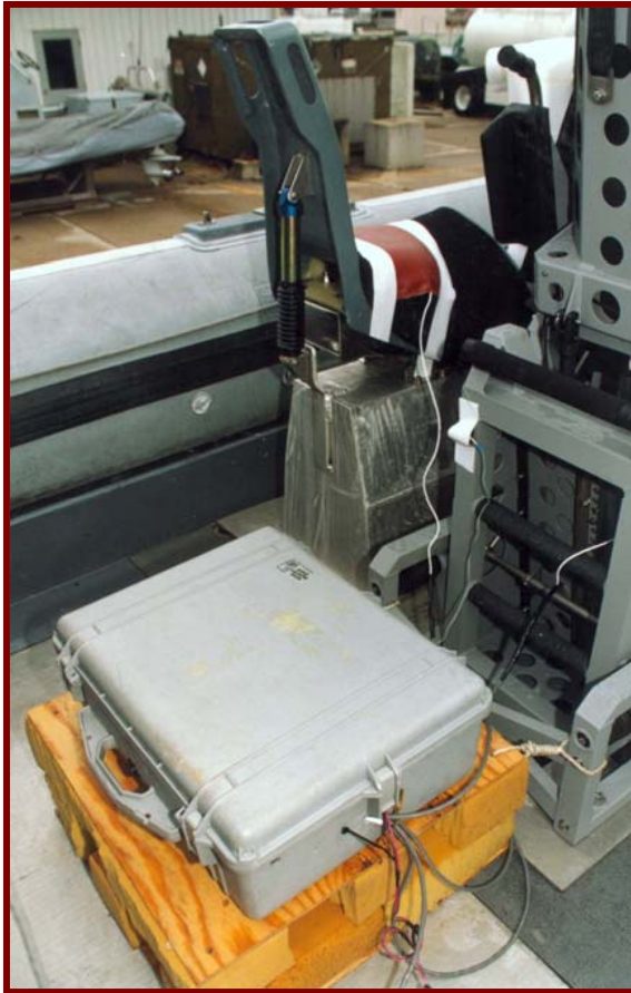
Laptop-Based Data Acquisition System Protected by Pelican Case and Foam Support
