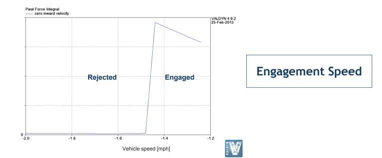
Following the DOE, additional analyses were performed to take a closer looks at the system dynamics and also evaluate the system's on hill engagement and disengagement performance. The maximum vehicle speed when parking on a hill was predicted to be 0.75 mph for both forward and reverse directions, which is less than the 1.44 mph engagement speed. Therefore, the vehicle will not roll away.
