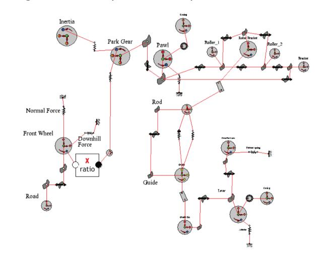
Park lock geometries are defined using VALDYN's LAMINA and LAMINAGEOM elements. The contact prosperities between each contact element are defined in the LAMINALINK element where contact stiffness, contact damping, and contact friction inputs are required.
