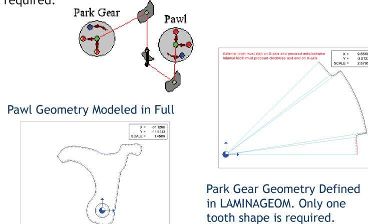
It may take many iterations to come up with a park lock design that meets all design requirements. Typically, the park gear's tooth width and tooth gap are adjusted to meet the engagement speed requirement. Spring forces can be adjusted as well. In this project, a design of experiment (DOE) approach is used to finalize the park gear geometry.
