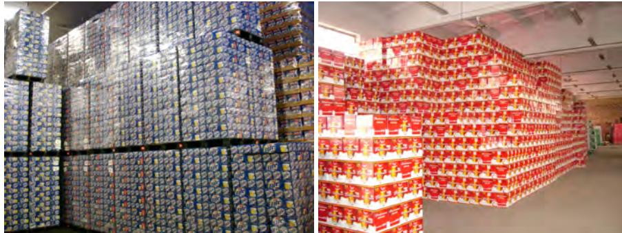
Figure 16.3: In the US warehouse on the left, cartons of beer have been palletized because labor is expensive compared to capital. The reduction in labor is worth the expense of a forklift plus the additional storage space. In the Chinese warehouse on the right, cartons have been stacked by hand and must be unstacked by hand; but labor is cheap and capital is expensive.
