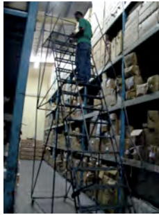
Figure 16.6: A ladder is much cheaper than a person-aboard truck, though much slower. (Note the product stored as loose cartons.)
