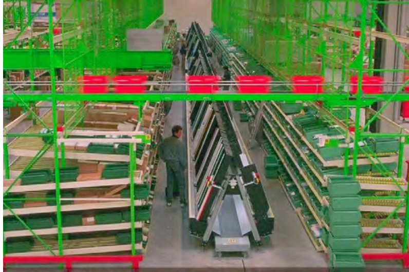
Figure 12.7: An A-frame automated item dispenser, as seen from the top (start) of the conveyor. The flow rack to either side hold product to restock the A-frame, and are in turn restocked from bulk storage.
