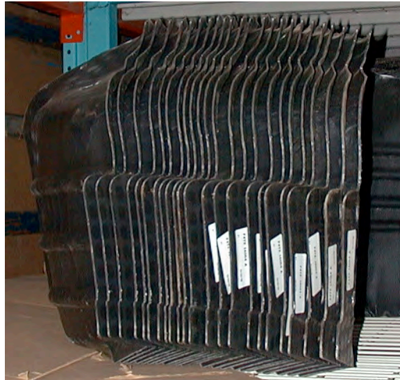
Figure 8.7: These plastic liners for the beds of pickup trucks nest like a set of spoons and so can be stored in little more space than that required by a single piece.
