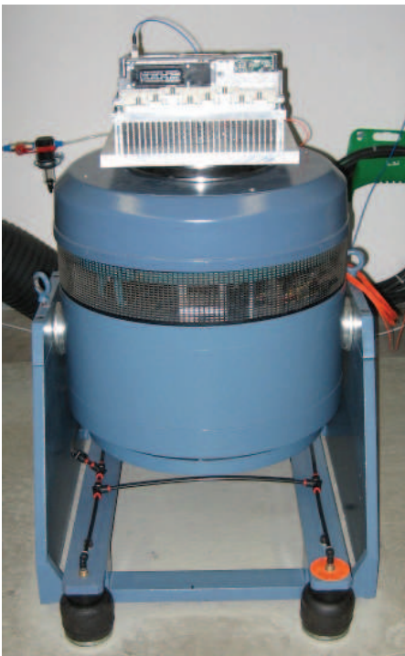
Figure 2.7.4 SKiiP system on a vibrating plate
