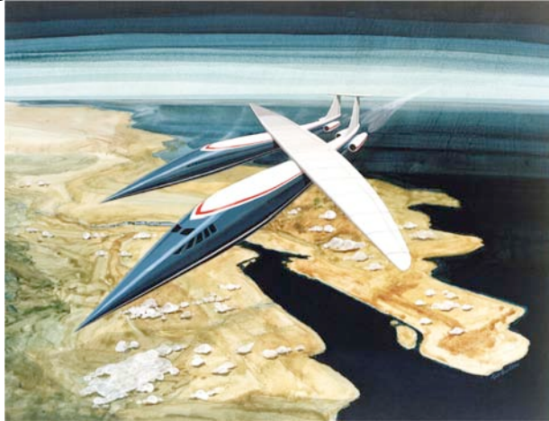
Figure 14. Twin fuselage oblique wing concept intended to reduce wing bending effects on structural loads and control.
