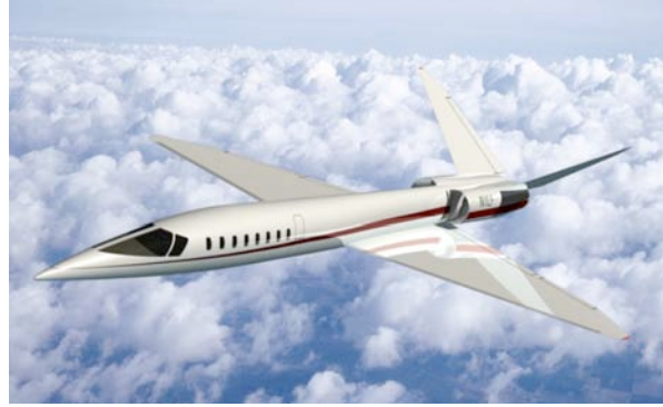
Figure 18. Artist concept of supersonic business aircraft with natural laminar flow wing. (Aerion Corporation)
