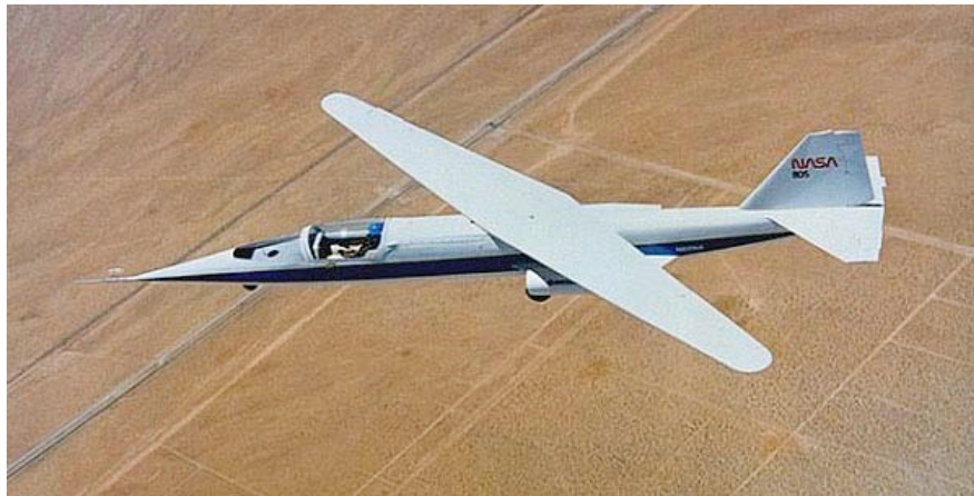
Figure 7. Oblique wing design (AD-1) tested by NASA in the early 1980's.
