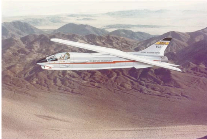
Figure 13. The oblique wing research aircraft concept was to utilize the digital flight control system of NASA's F-8 aircraft.
