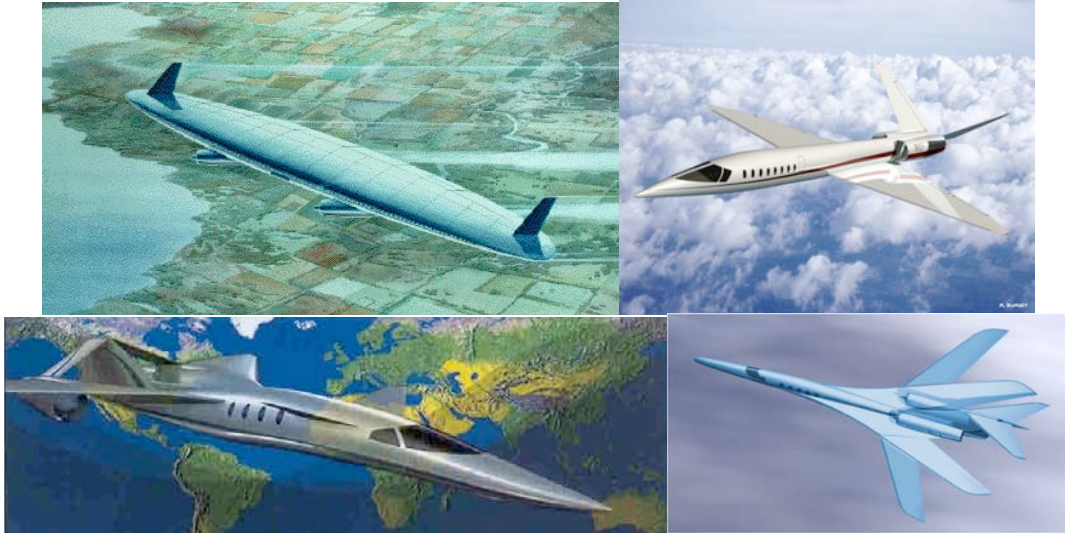
Figure 4. A variety of unconventional designs proposed for efficient supersonic flight.
