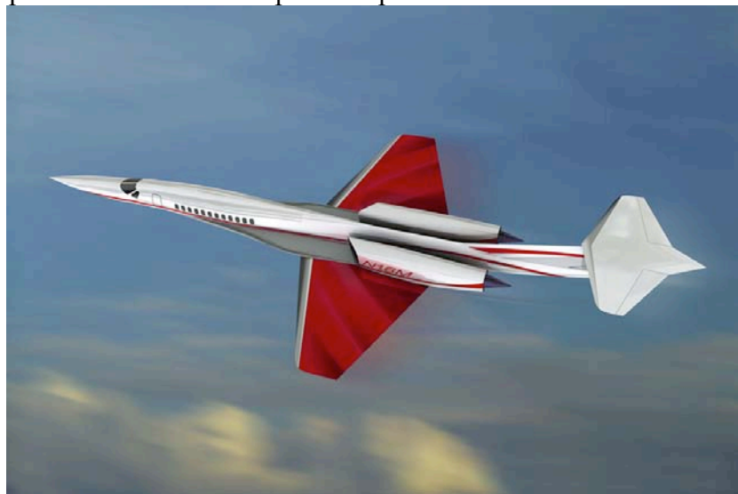
Figure 27. Aerion supersonic laminar flow concept.
