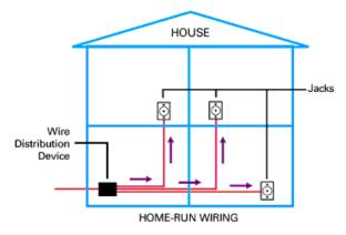
You may find a combination of these strategies where there is a continuous loop on a floor of a house, but each floor feeds independently to the demarcation point. In older condo and apartment buildings you are likely to find a continuous loop, but newer buildings incorporate the "home run" method.
