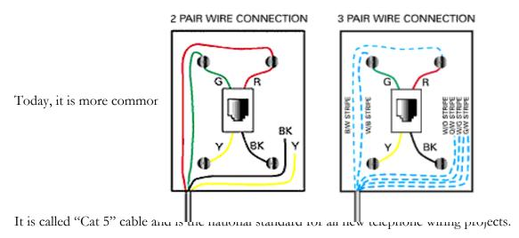
3. Fasten the jack casing securely to the wall or baseboard using the appropriate metal or wood screws. Pull the wire through the opening in the jack casing and connect it as depicted here:
