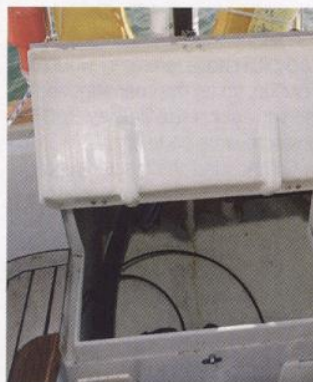
Gigi's lazarette, hinged at the coaming rather than the seat, can handle larger bits of kit
