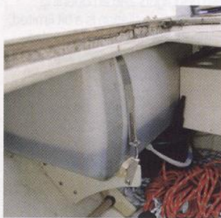
Rogers has fitted Gigi with a plastic fuel tank, easily accessible from the big cockpit locker to port
