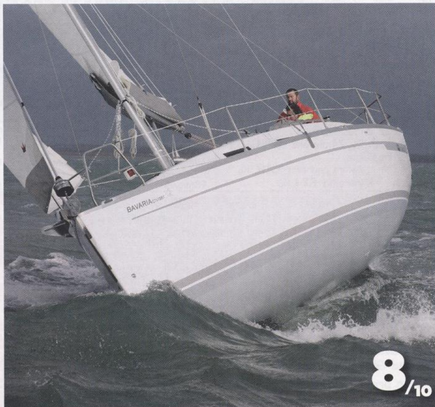
The Bavaria's sailplan scored with power shared more evenly between mainsail and jib
