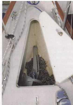
The shallow anchor locker is big enough for an 11kg (25 lb) CQR and 50m of 6mm chain
