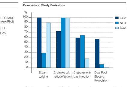
Fig. 2 Comparative emission levels from various LNG propulsion types
