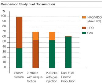
Fig. 1 Fuel consumption relative to steam turbine system (100%)
