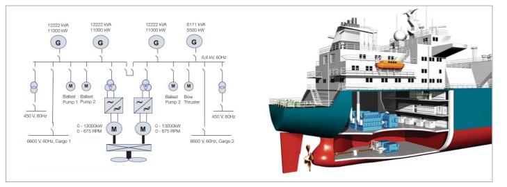
Fig. 4 Typical configuration for a single skeg LNG Carrier
