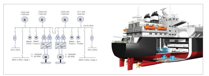
Fig. 5 Typical configuration for a twin skeg LNG Carrier
