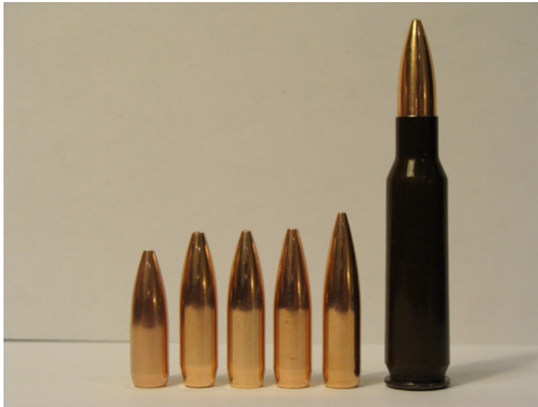
6mm/.243 (L-R) Sierra 70gr MK, Sierra 85gr HPBT, Sierra 90gr FMJBT, Hornady 87gr BTHP, Berger 90gr Match Target, 6.2mm OCC with Sierra 90gr FMJBT.
