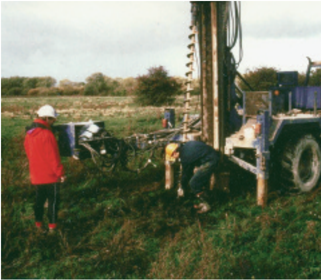
Augering of palaeochannel deposits in Trent Valley near Shardlow, Derbyshire (photograph: D. Knight)
